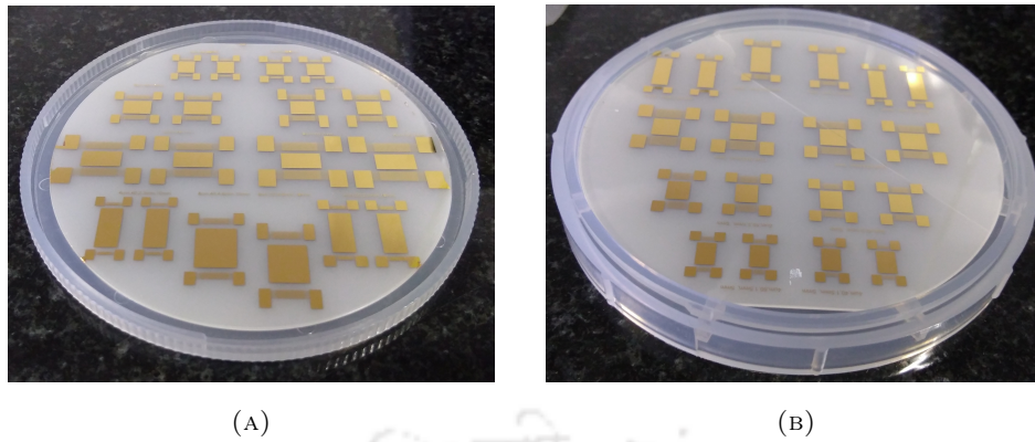
FIGURE 3.5: Final devices after lift-off on: (A) 41^\circ\text{YX LiNbO}_3 , (B) 36^\circ\text{YX LiTaO}_3
