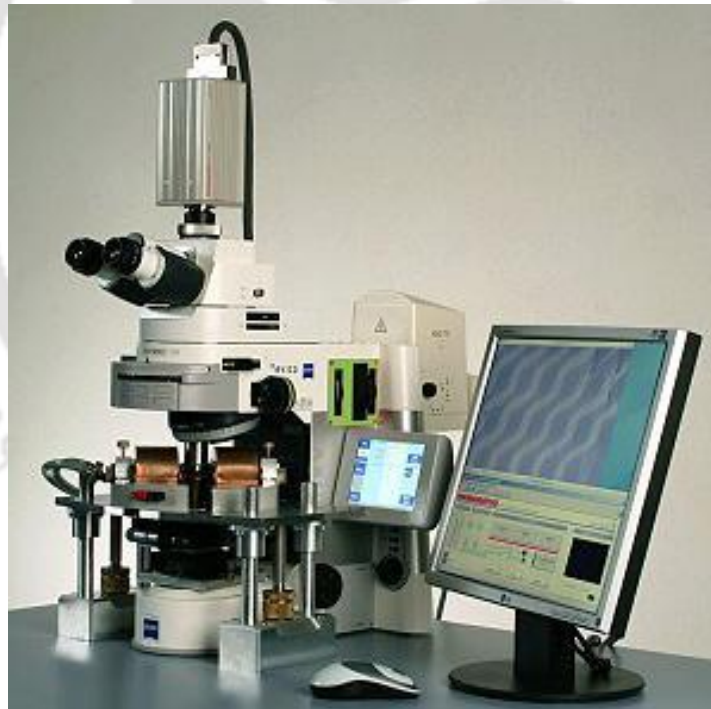
Figure 3.15: Photographic view of the Kerr microscope (Evico Magnetics Ltd. Germany) used in the present study.
