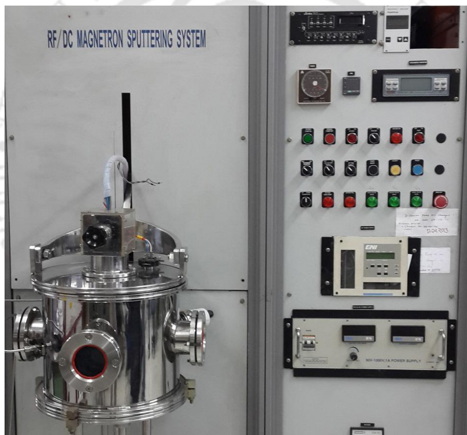
Figure 3.04: Photographic view of the magnetron sputtering system used in the present work.
