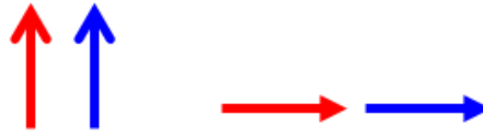
Figure 2.08: Schematic drawing of broadside and head-to-tail configurations for a pair of ferromagnetically coupled magnetic moments.
