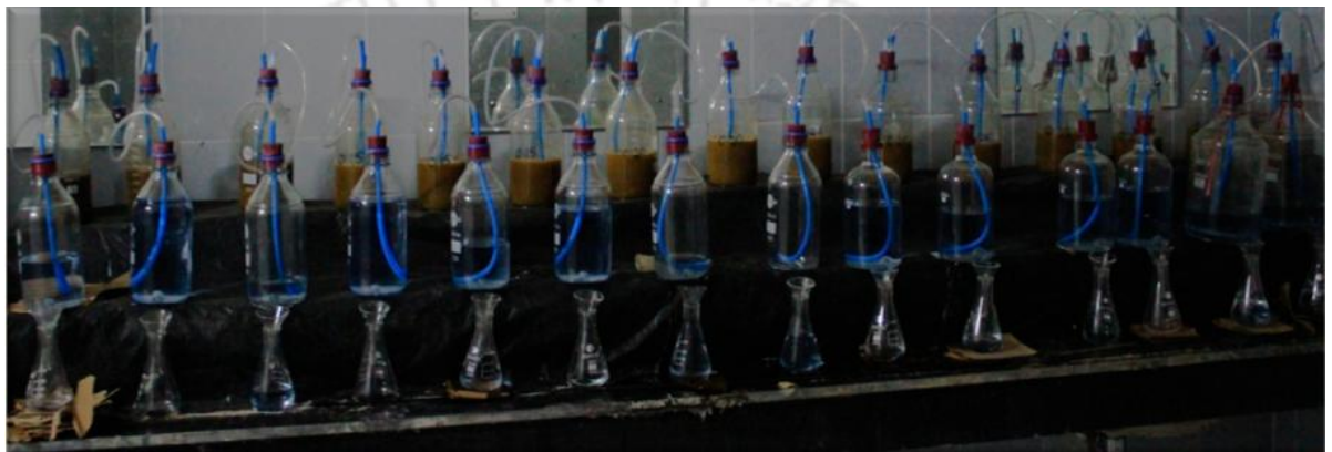
Fig. 3.3 Schematic diagram and Anaerobic batch setup with different F/M ratios
