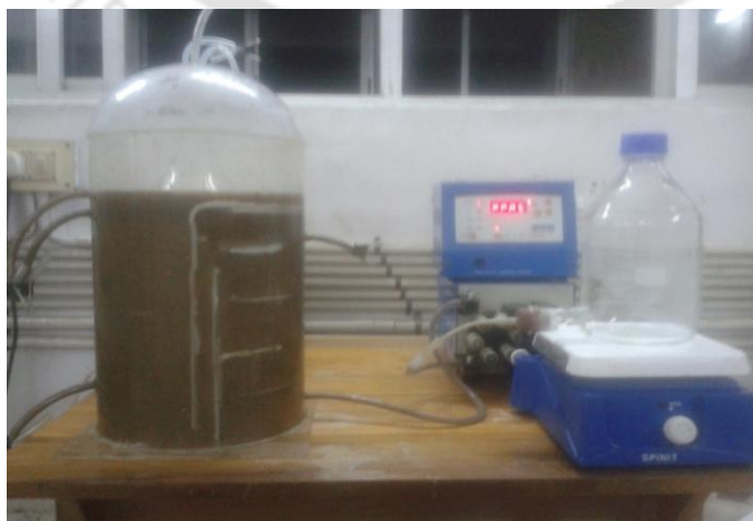
Fig. 3.7 Schematic and pictorial view of continuous anaerobic digester
