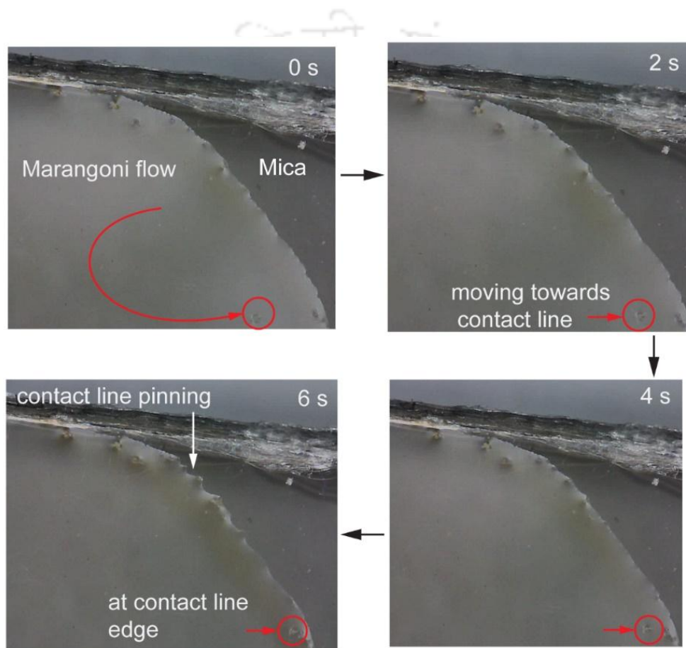
Figure 2.9. Digital microscope images of droplets showing Marangoni flow [1] of \text{Na}_2\text{PdCl}_4 particles with heating at 50^\circ\text{C} on a hotplate (on a cleaved mica surface); the red circle illustrates the direction of the flow within the droplet. With time, \text{Na}_2\text{PdCl}_4 particles move towards the contact line and reach the contact line after 6 seconds of heating.
