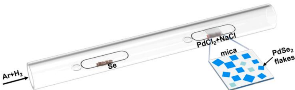
Figure 1.9. Schematic showing the NaCl assisted Synthesis of PdSe 2 flakes on mica substrate by APCVD. (Adopted from Ref 39 )
