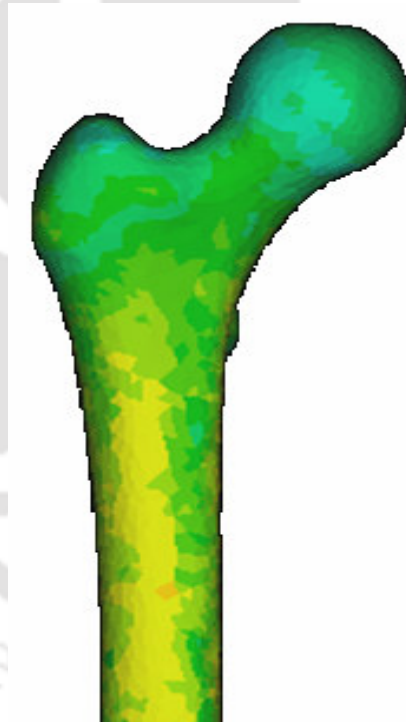
Figure 6.2: Finite element model of femur bone with distribution of Young's modulus.
