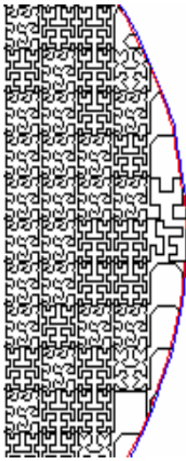
Figure 5.6: A small region zoomed up to show the LM tool path for HA scaffold.
