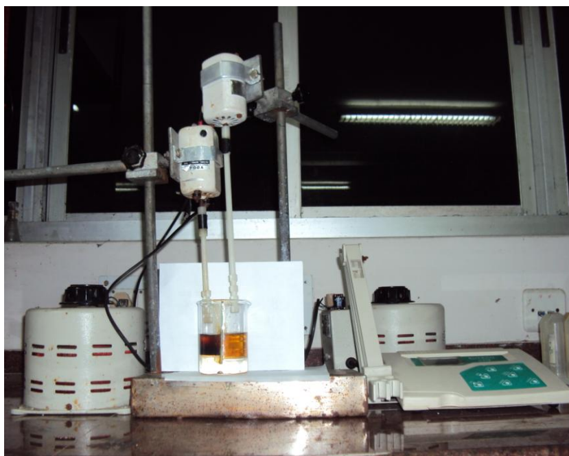
Figure 2.3 Photograph of BLM set-up
