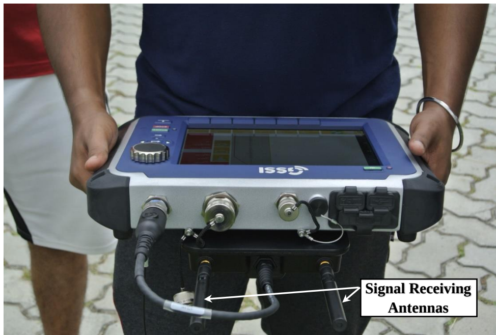
Figure 6.7: Display and control unit of GPR
