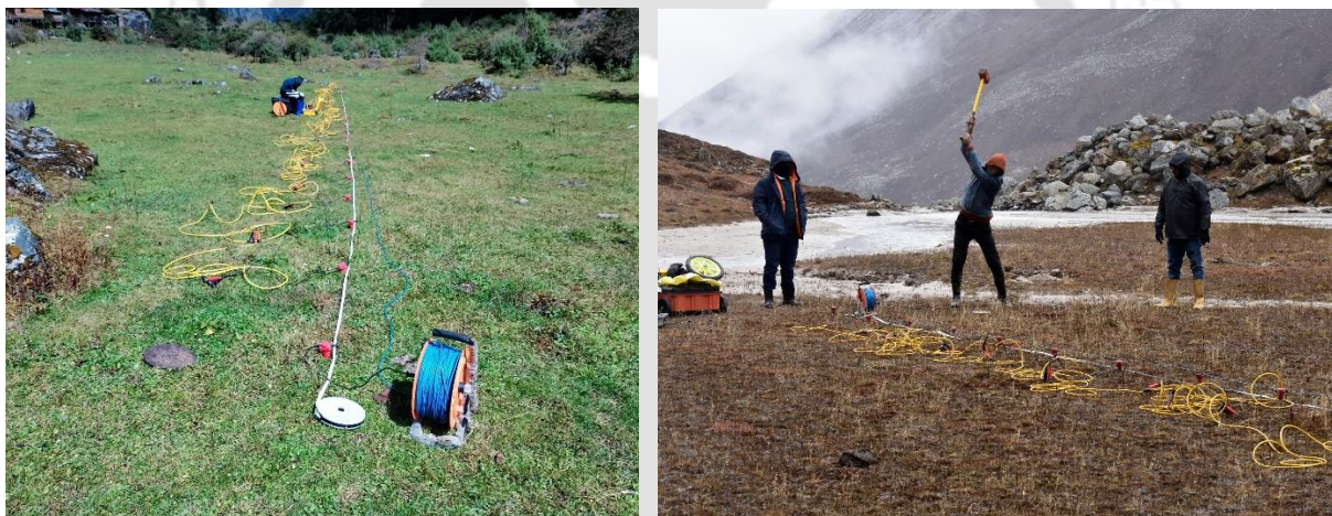
Figure 6.8: MASW survey at a location (MASW5) between Lachen and Thangu valley (left) and (MASW2) Changme glacial snout (right)
