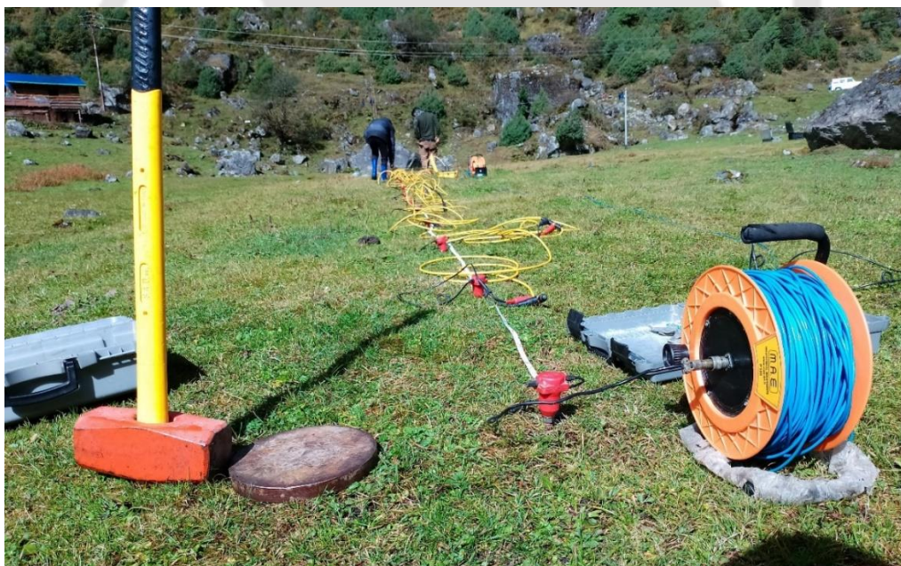
Figure 6.4: Installation of MASW geophones for data acquisition
