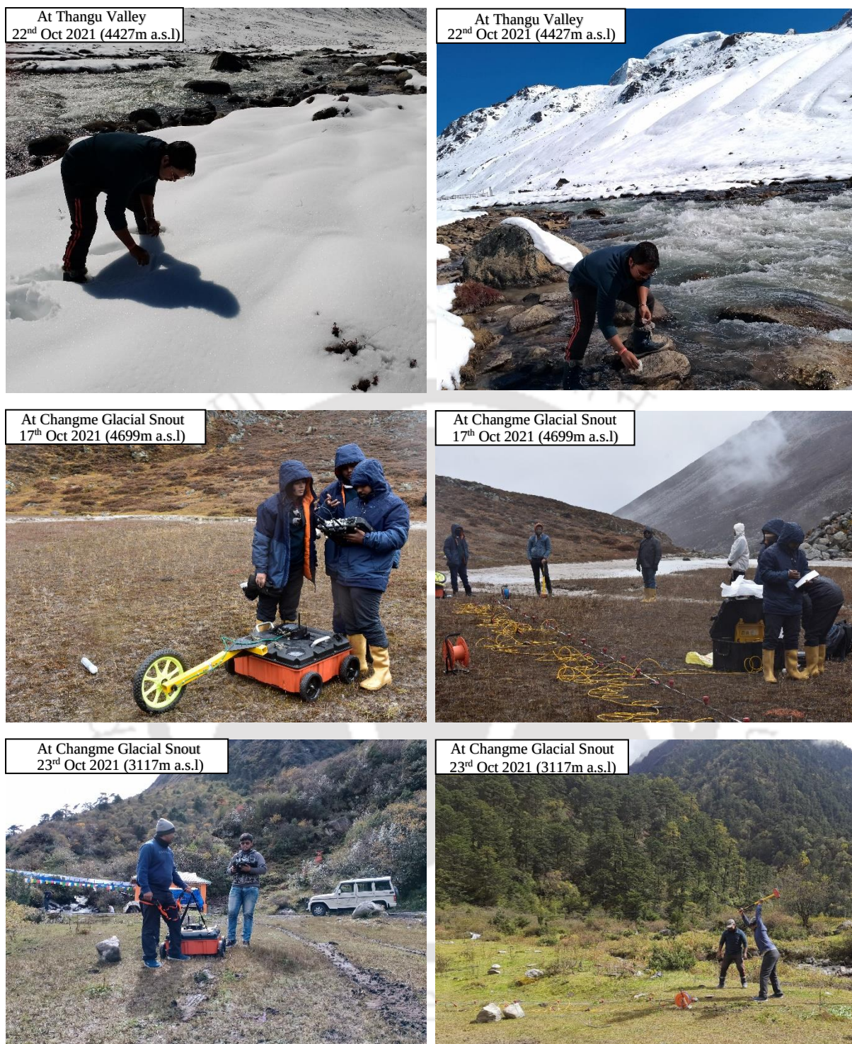
Figure A.4: Field investigation-III photographs of collecting water and snow samples, GPR and MASW survey
