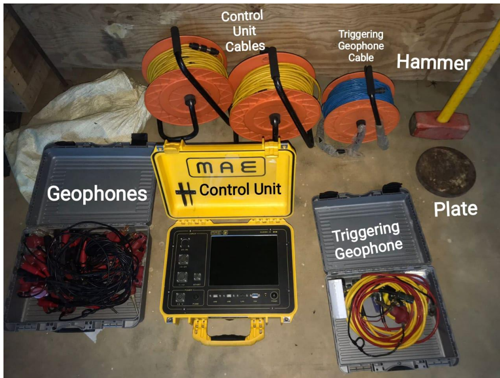
Figure 6.3: MASW survey kit with all the components
