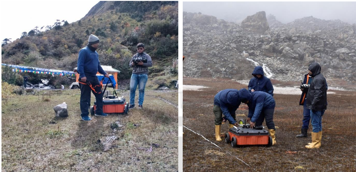
Figure 6.16: GPR survey at a location (MASW5) between Lachen and Thangu valley (left) and (MASW2) Changme glacial snout (right)
