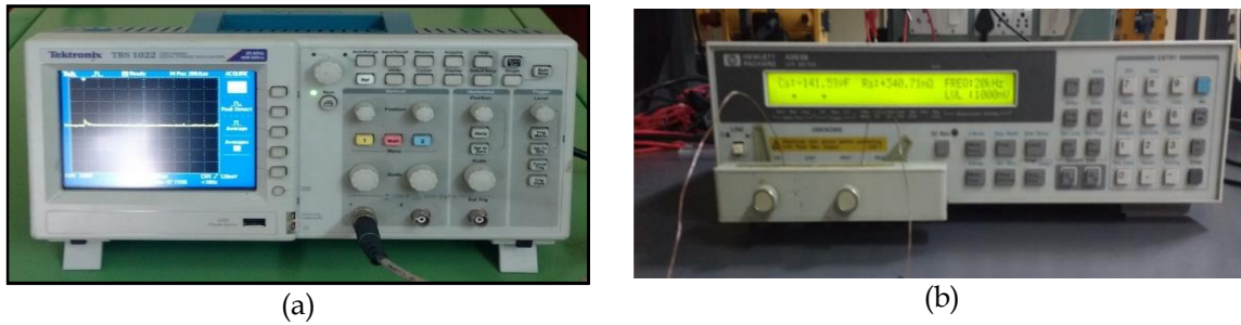
Figure 3.25 (a) Oscilloscope for current measurement and (b) RLC measuring equipment
