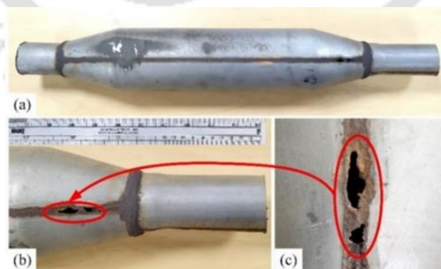
Figure 8.1 (a) Muffler, (b, c) Failure at the weld zone
