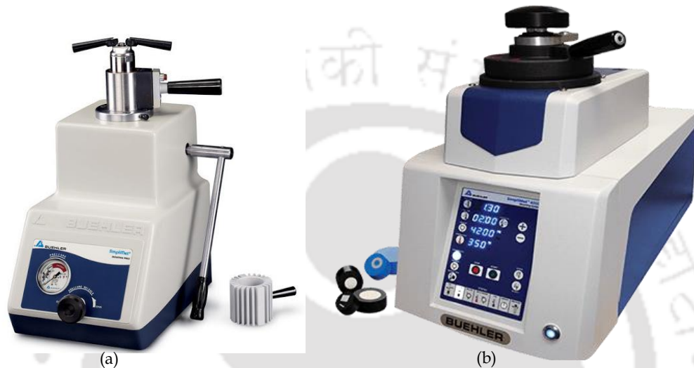
Figure 3.26 Metallographic specimen molding unit (a) Manual and (b) Automatic
