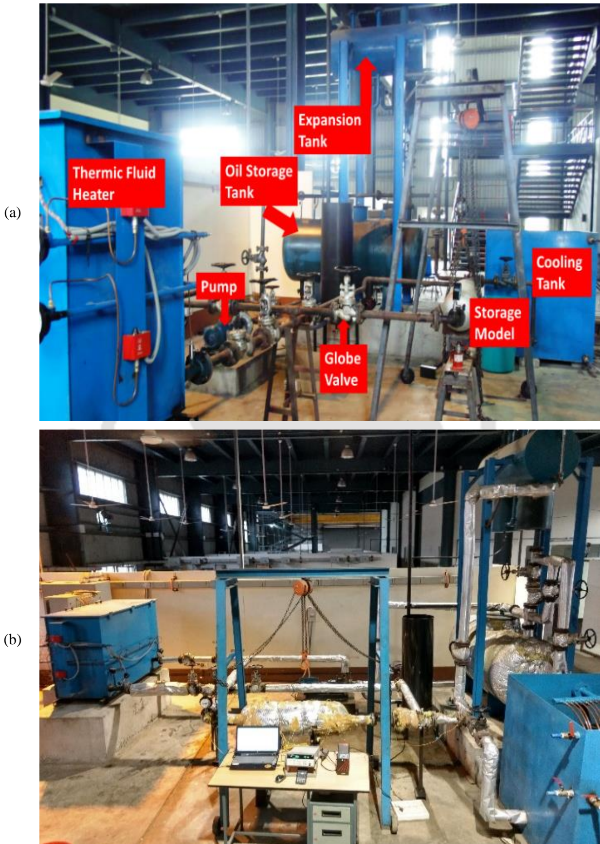
Fig. 4.2 Pictorial view of the experimental setup (a) without insulation (b) with insulation.
