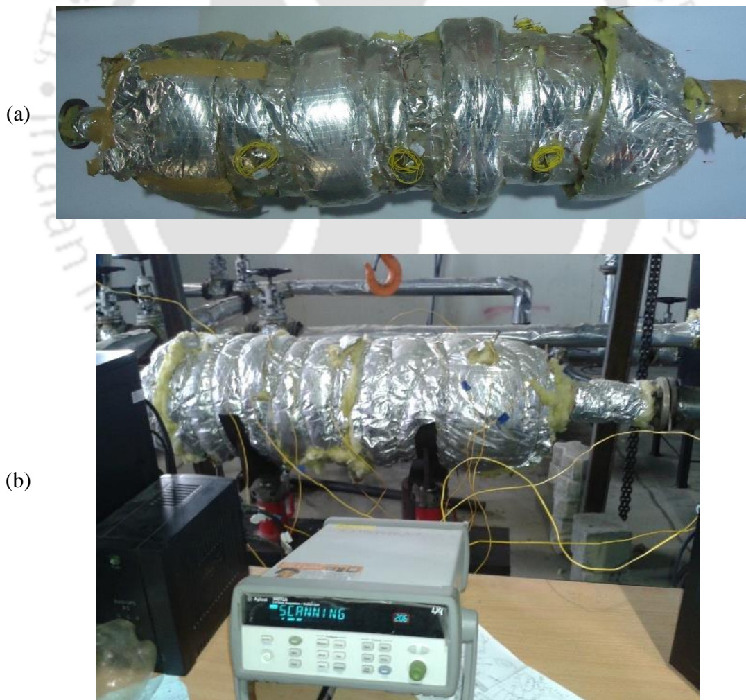
Fig. 4.5 Pictorial view of the LHS prototype (a) with thermocouples (b) during experiments.
