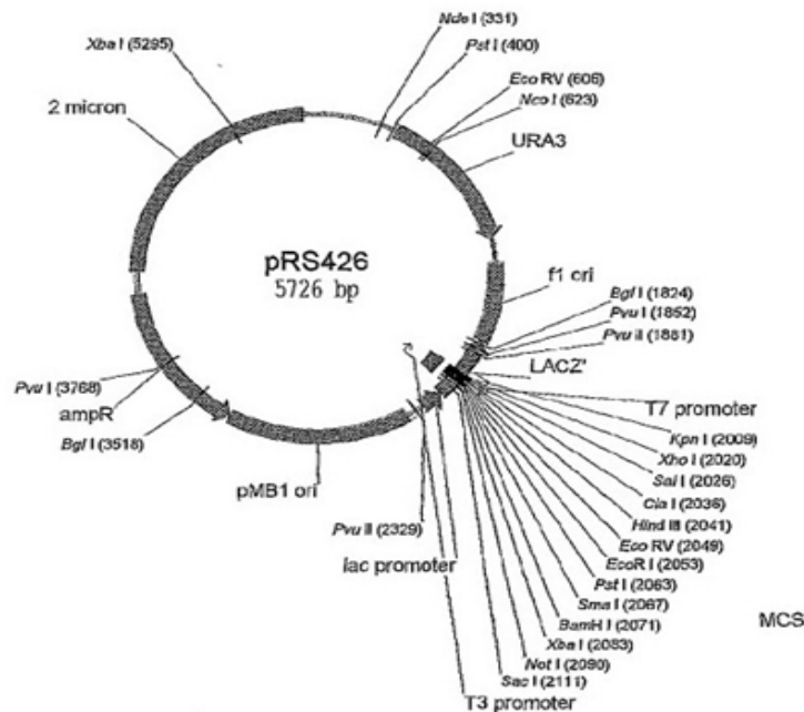
Figure 2.2: Schematic of the pRS426 vector. The size of the vector is 5.726 kb. The unique restriction sites are SacI BstXI SacII EagI NotI SpeI BamHI SmaI EcoRI HindIII ClaI SalI XhoI KpnI are present in the polylinker region of lacZ' sequence. The URA3 , an auxotrophic marker for selection in S. cerevisiae , and amp R marker for selection in E. coli through blue-white screening. The plasmid map is available at http://www.creative-biogene.com/pRS426-phagemid-in-E.-coli-vector-VET1104-179-16.html .
