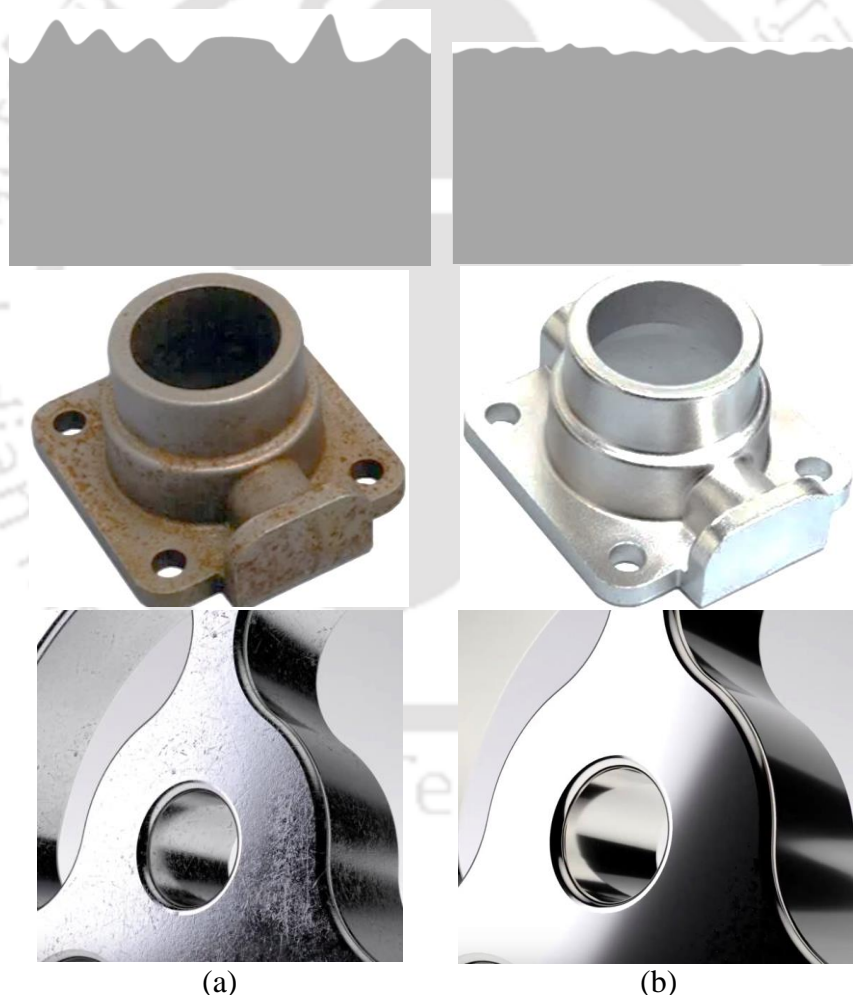
Fig. 1.3 Surface conditions (a) before and (b) after EP [6], [7]
