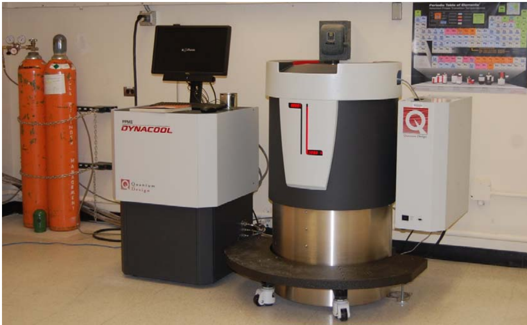
Figure 3.19: Photographic view of a PPMS system with cryogen free option.
