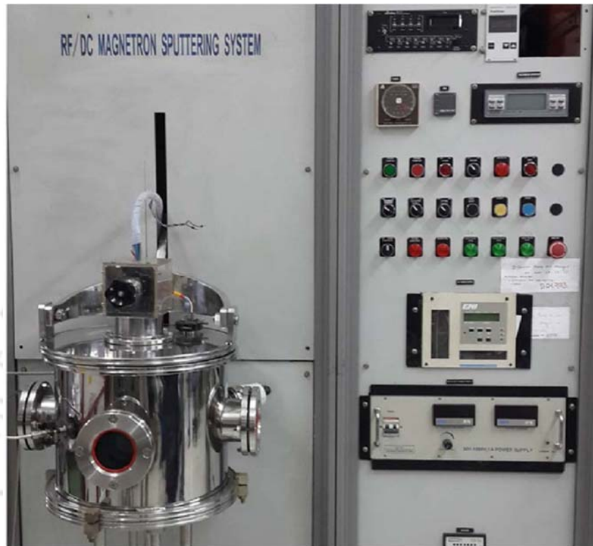
Figure 3.05: Photographic view of the magnetron sputtering system used in the present work.
