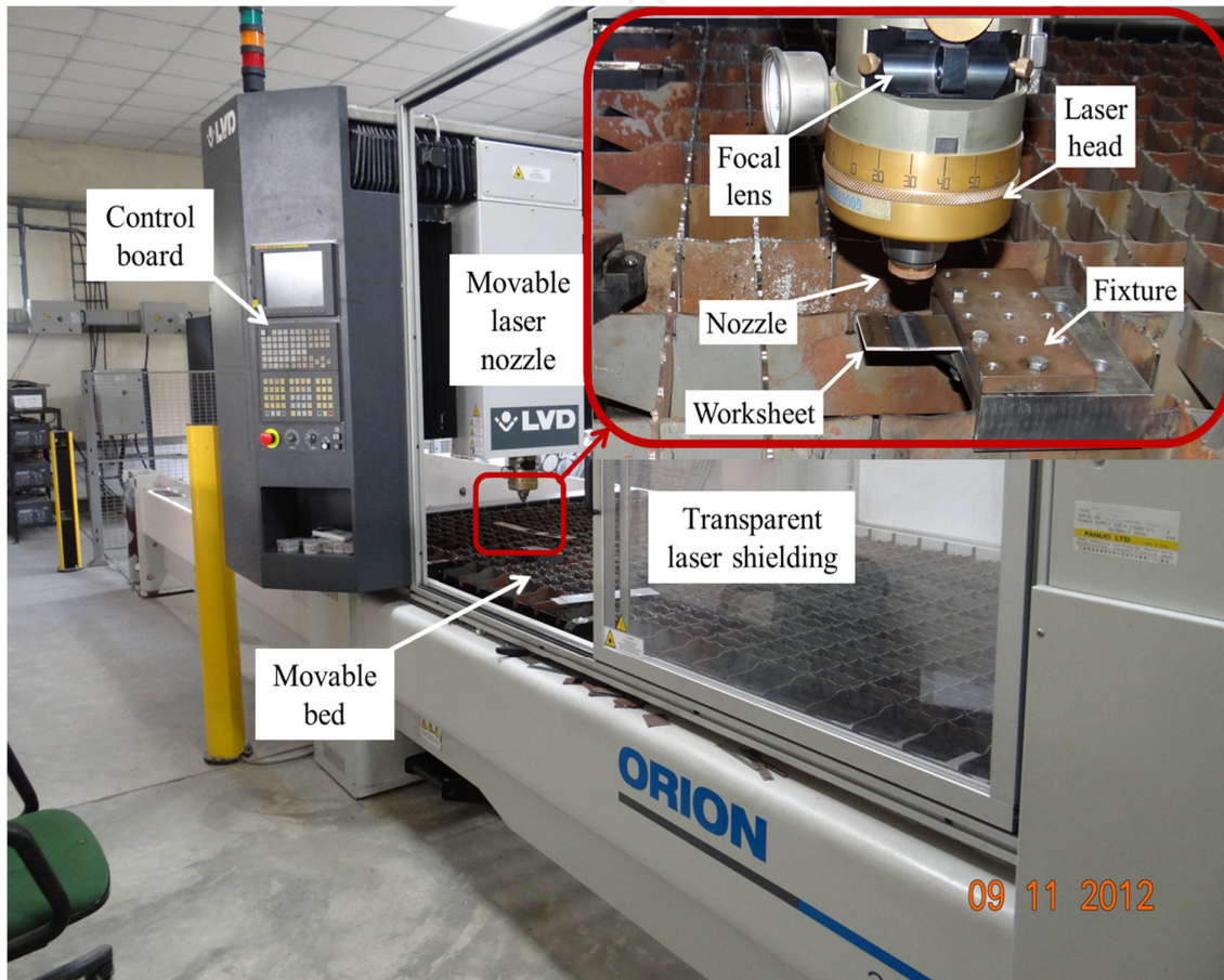
Figure 3.3. Details of laser machine setup.
