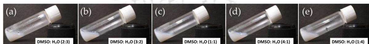
Figure A6.2: Gelation study of Py-H in DMSO: H 2 O ratio of (a) 2:3, (b) 3:2, (c) 1:1, (d) 4:1, (e) 1:4, and (e) 1:4.
