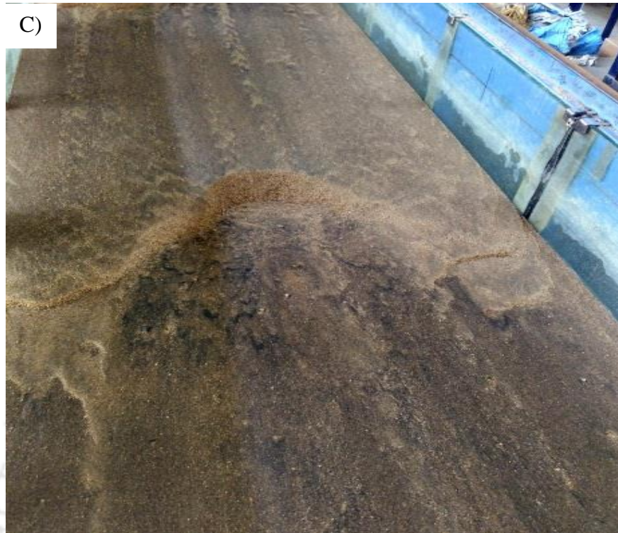
Figure 3.15 Snapshot of channel for A) Shape-III, B) Shape-IV and C) Shape-V after distortion of bank profile.
