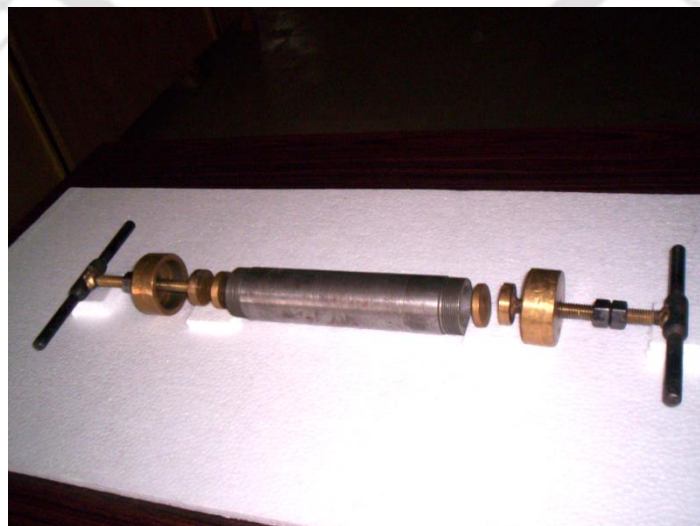
Fig. 3.9 Fabricated miniature static compaction tool
