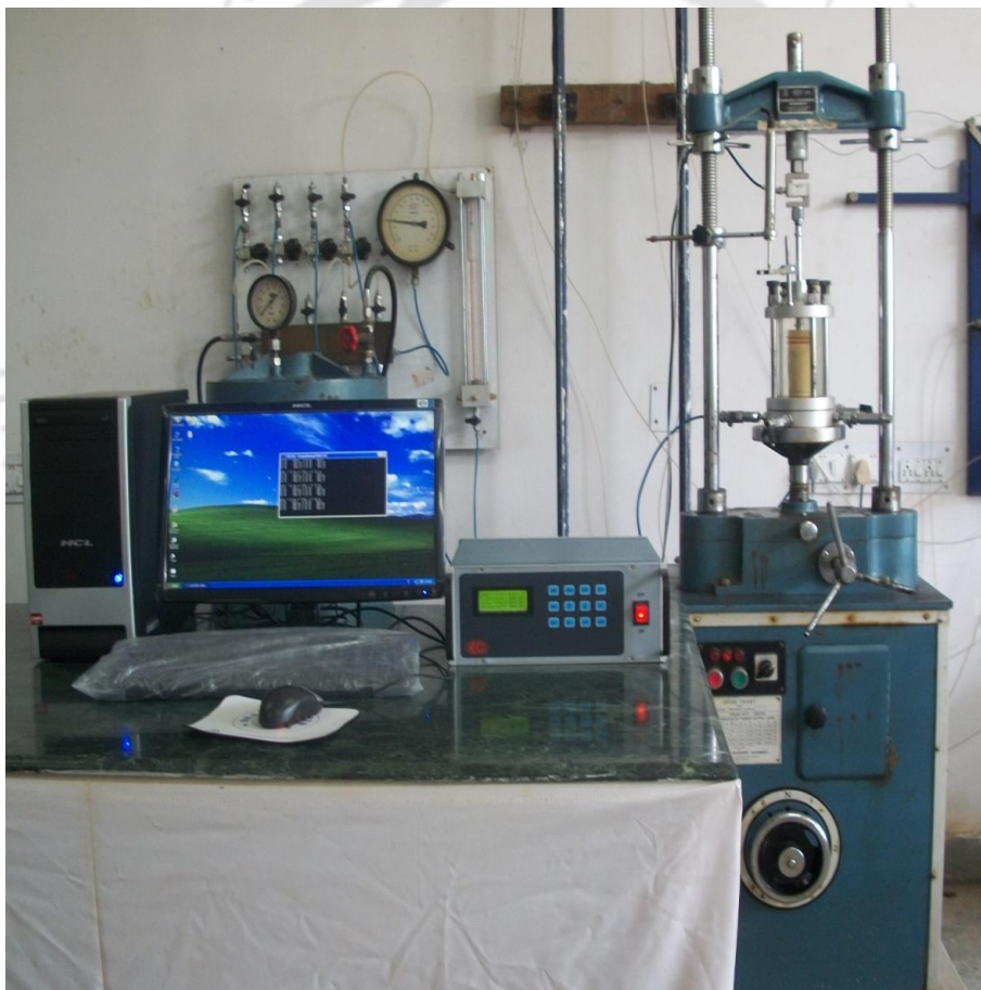
Fig. 3.8 Electronic triaxial set-up
