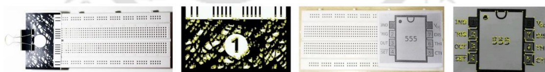
Figure E4. Different types of breadboard markers used with our AR prototype and their tracking features, shown in yellow, stored in image target database. These features are tracked as long as the image is at least partially in the camera’s field of view.
