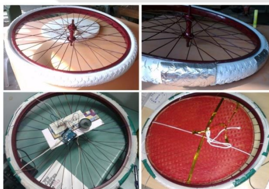
Figure 2. Round Piano prototype showing Arduino board mounted at the center to allow rotation of the wheel with touch-sensitive aluminum foils on the sides.
