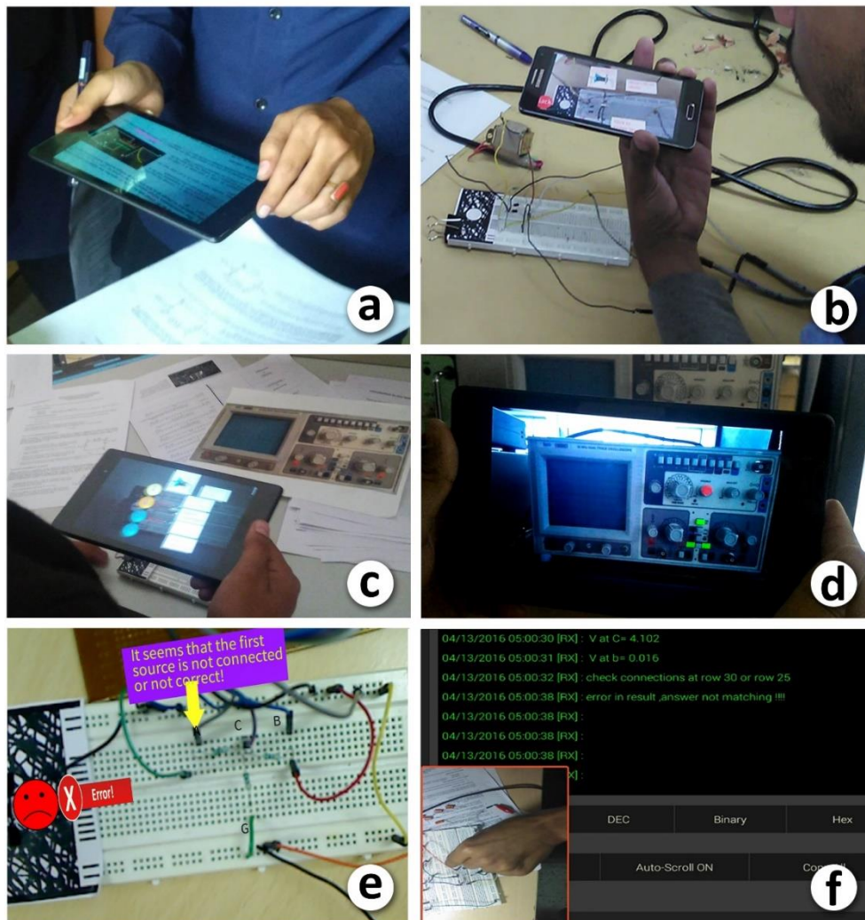
Figure 5.4 Augmented Reality and intelligent breadboard. (a) Video instructions overlaid on a lab manual, (b) Breadboard attached with marker, (c) Close-up view of the 3D graphics overlaid on a breadboard, (d) Operating instructions for CRO, (e) AR based instructions provided by intelligent breadboard on a computer screen. The exact location of mistakes or errors committed by users on the breadboard are pinpointed via AR, (f) Snapshot of instructions provided by intelligent breadboard on digital tablet.
