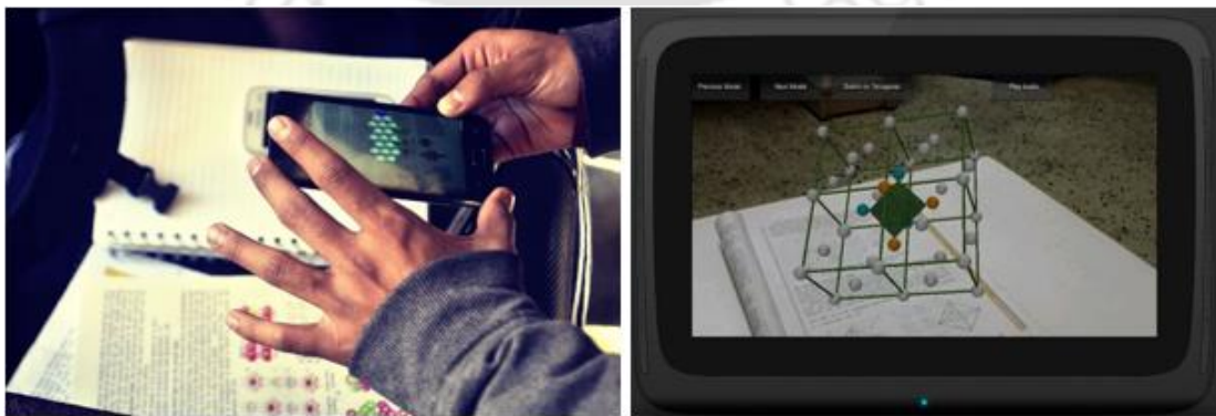
Figure 1.6 A view of Augmented Reality on a mobile device. Virtual objects, in the form of 3D graphics, overlaid on a real-world environment. Source: (Amrit, Bansal, & Yammiyavar, 2015)
