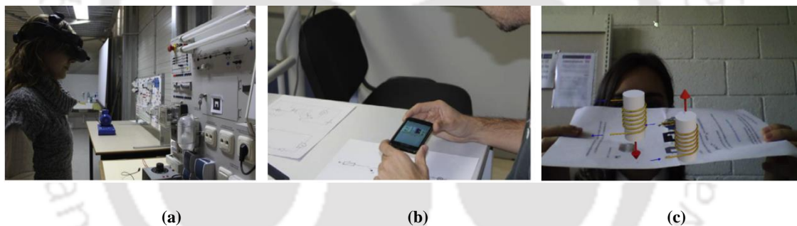
Figure 2.7 Augmented Reality for electrical engineering. (a) A head-worn device utilizing marker based image tracking to display 3D content to students regarding equipment operation. (b) and (c) Content such as 3D images are shown when the mobile device is pointed towards lab manuals. Image Source: (Martín-Gutiérrez, Fabiani, Benesova, Meneses, & Mora, 2015)
