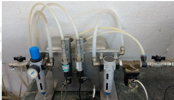
(b) Dry air receiver unit
