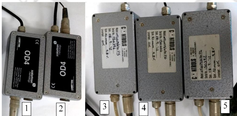
(b) Data logger for (1) actuator (2) external LVDT (3) on-sample LVDT1 (4) on-sample LVDT2 (5) on-sample LVDT3
