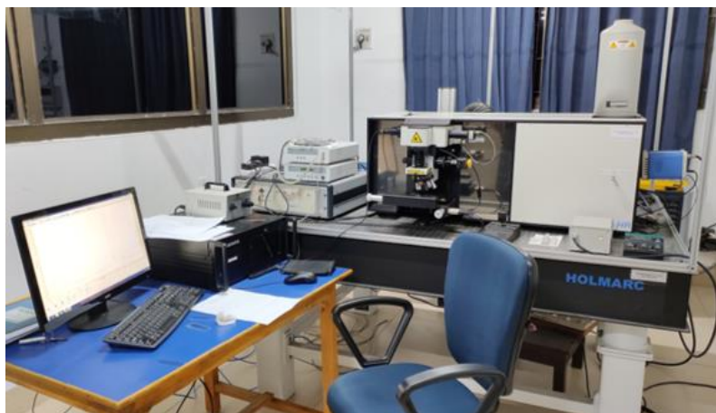
Figure 2.12: Photograph of Raman spectrometer (LBRAM HR800).
