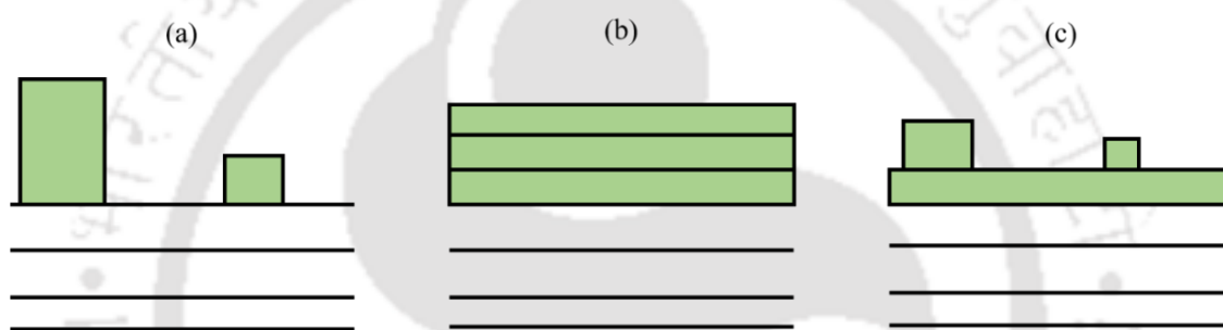
Figure 2.6: Different growth modes in thin film deposition, (a) Volmer-Weber growth, (b) Frank – van der Merwe growth and (c) mixed growth.
