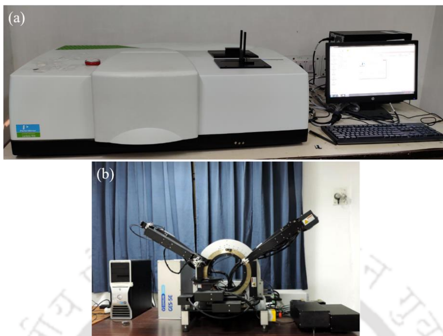
Figure 2.25: (a) Photograph of UV-VIS-NIR spectrophotometer and (b) Spectroscopic ellipsometer.
