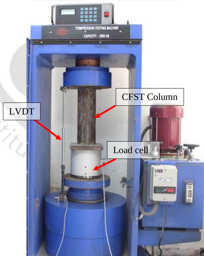
Figure 4.2 Circular CFST under compression
