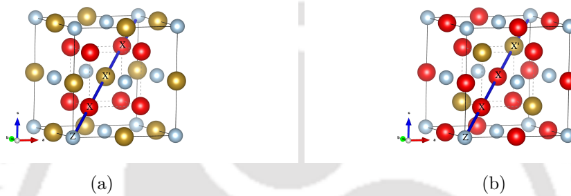
Figure 3.1: Crystal structure of ternary Heusler compounds X_2X'Z in (a) T_I (Heusler i.e two X atoms are in symmetric positions) (b) T_{II} (Inverse Heusler i.e X and X' are in symmetric positions).
