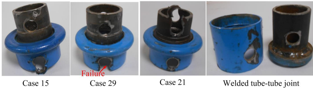
Fig. 3.17 Failure pattern of different end formed cases and welded tube-tube joint during destructive pull out test
