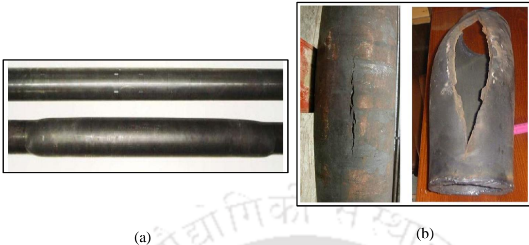
Figure 2.1 Photographs of (a) original and ballooned pressure tube[27] and (b) failure in power plant pipe due to creep[28].
