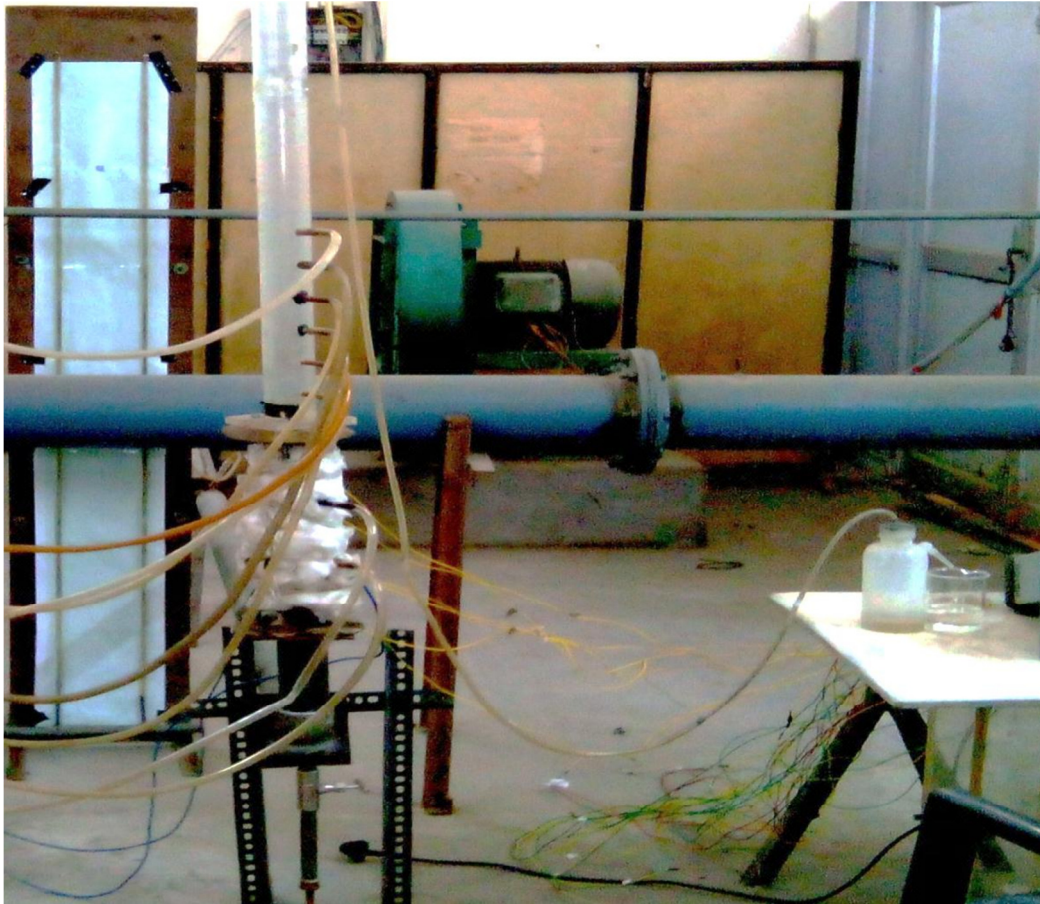
Fig 5.3 Photograph of experimental setup for CO 2 adsorption in fluidized bed
