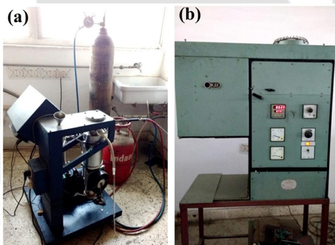
Figure 2.07: Photographs of (a) ampoule sealing setup, and (b) raising hearth furnace.
