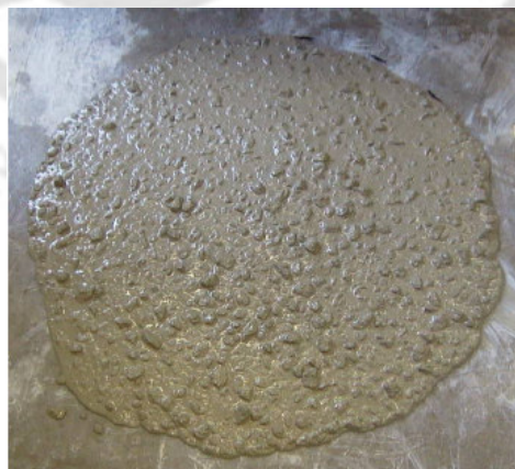
Fig 3.2 No segregation after slump flow
