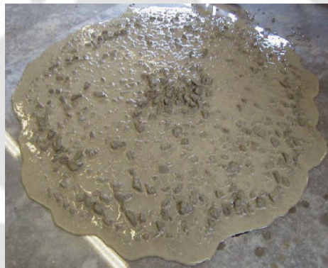
Fig 3.4 Segregation due to large mortar halo and aggregate piling at centre
