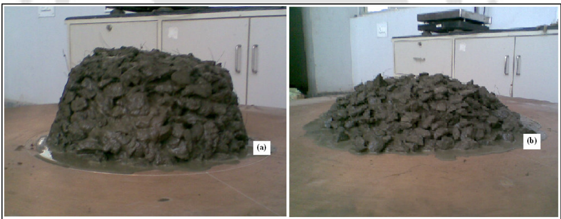
Fig 4.20. Flow test of FRC (a) After lifting the cone (b) After jolting the flow table
