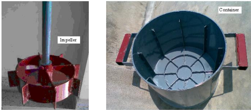
Fig 2.2 (a) Impeller (b) Cylindrical container of present rheometer
