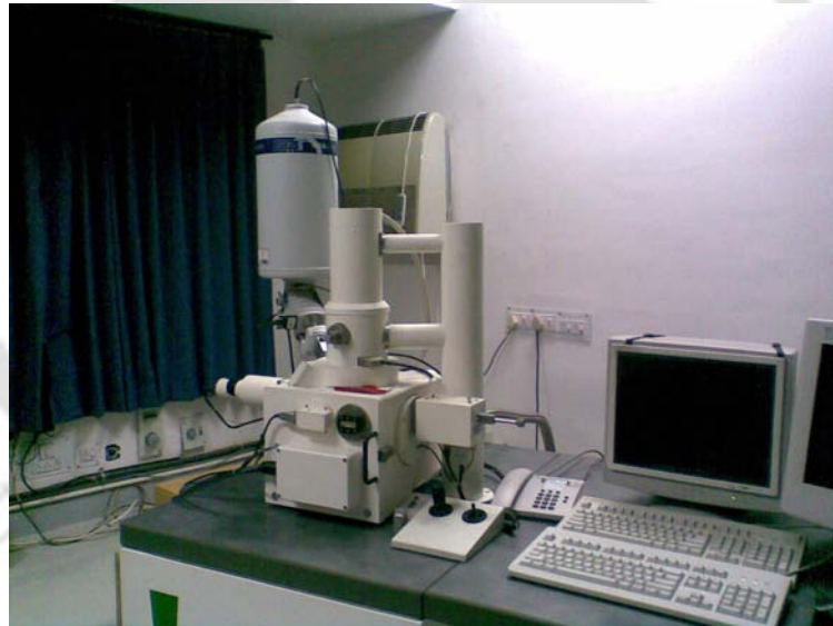
Fig 4.2. Scanning electron microscope used in the present study
