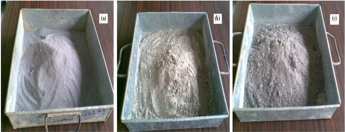
Fig 4.1. Mineral admixtures used in the present study (a) Condensed silica fume (b) Fly ash (c) Rice husk ash
