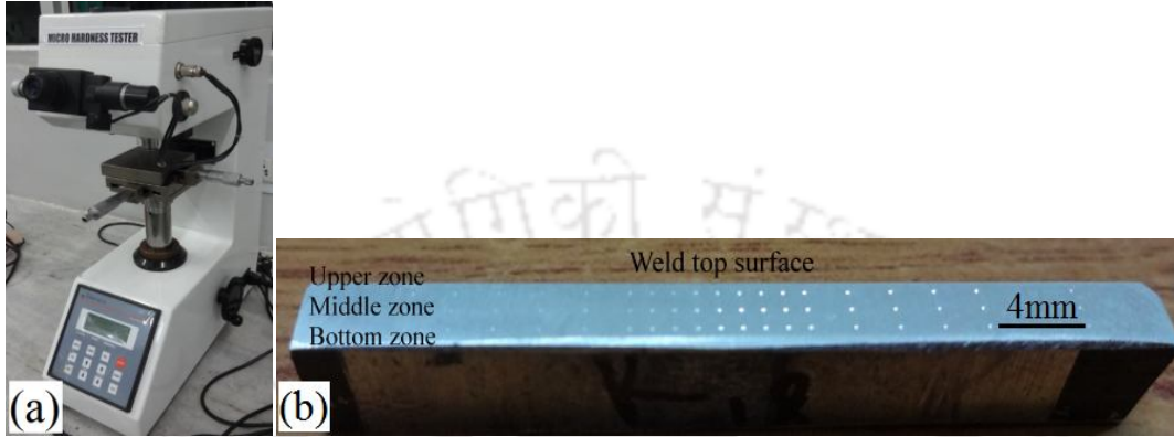
Fig.3.11 (a) Vickers micro-hardness measuring machine, (b) hardness specimen with indentation marks
