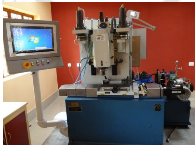
Fig.3.4 FSW setup used for Al/Cu dissimilar welding
