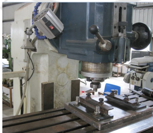
Fig.3.1 FSW setup used for the experiment
