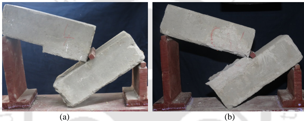
Fig. 3.13. Tension bond failure in Z-shaped specimens at: (a) top brick and mortar joint; and (b) mortar joint and bottom brick.
