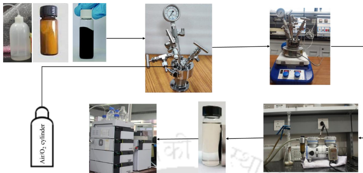
Figure 2.3: Schematic representation of experimental setup for oxidation reactions.
