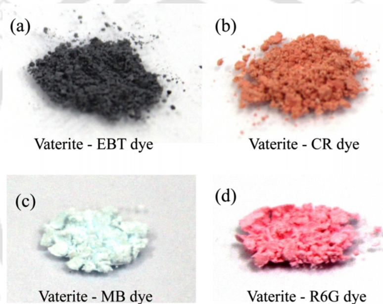
Figure 6.19. Image of the dye loaded vaterite particles, (a) EBT loaded vaterite, (b) CR loaded vaterite, (c) MB loaded vaterite and (d) R6G loaded vaterite.
