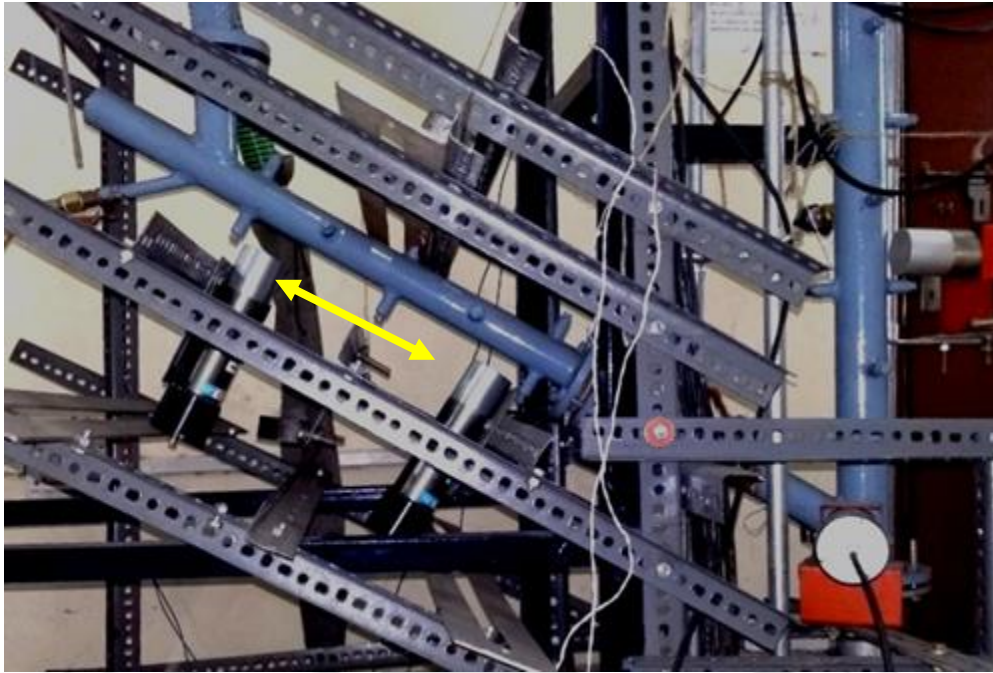
Figure 3.3 Photograph showing the detector position for RTD measurements (Lead sheets are removed for the sake of clarity)
