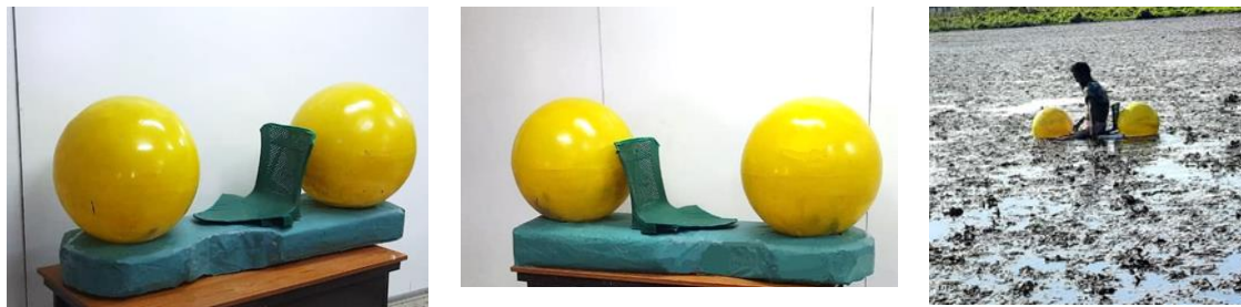
Figure 26. Alpha prototype of the floating device and its field-testing
