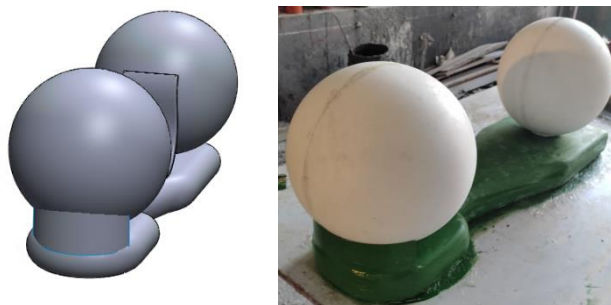
Figure 29. Iterations in the prototype (covering front gap)
