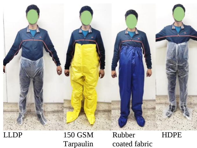
Figure 51. PPE developed with different materials
