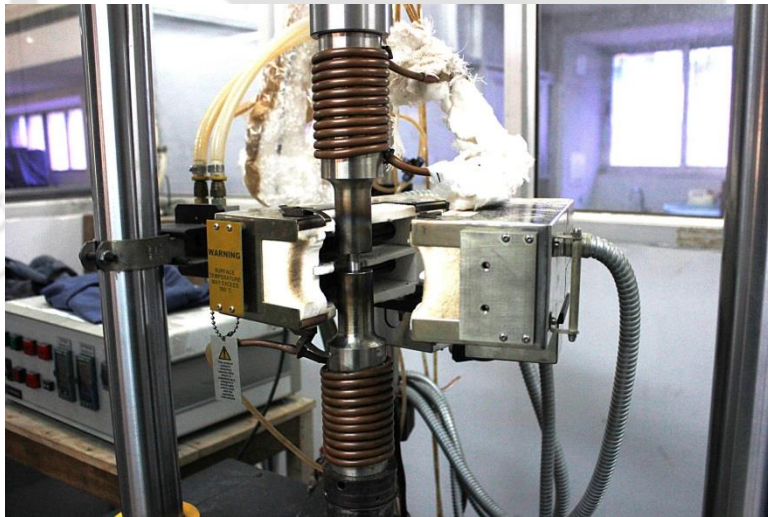
Figure 3.14 Photograph of the high temperature compression testing setup
