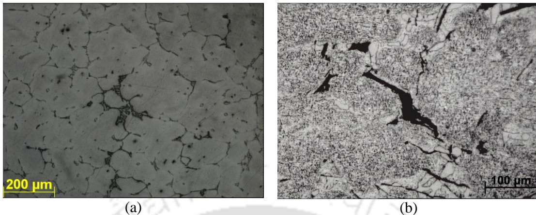
Figure 4.45 Optical micrograph of Alloy-B (a) before hot deformation (X10 magnification) and (b) void formation at triple junctions (X20 magnification) at strain rate 1 \text{ s}^{-1} and temperature 300 \text{ }^\circ\text{C}
