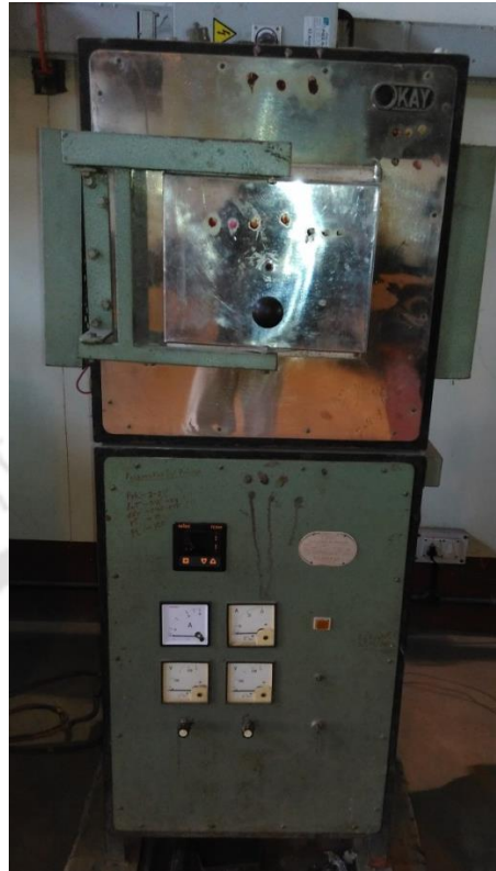
Figure 3.5 Photograph of the muffle furnace used for heat treatment
