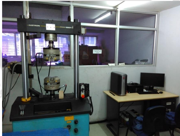
Figure 3.13 Photograph of 100 kN capacity servo-hydraulic controlled dynamic universal testing machine
