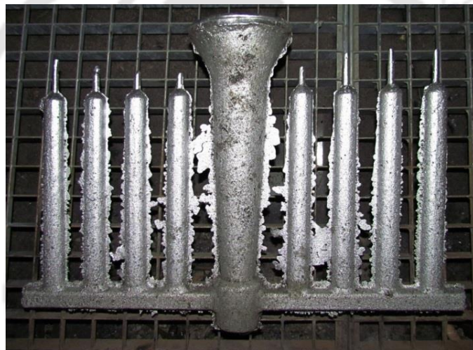
Figure 3.2 Photograph of the alloy after sand casting
