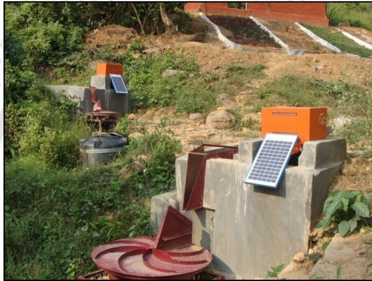
Figure 4.6: The sediment and runoff sampler located at the experimental watershed
