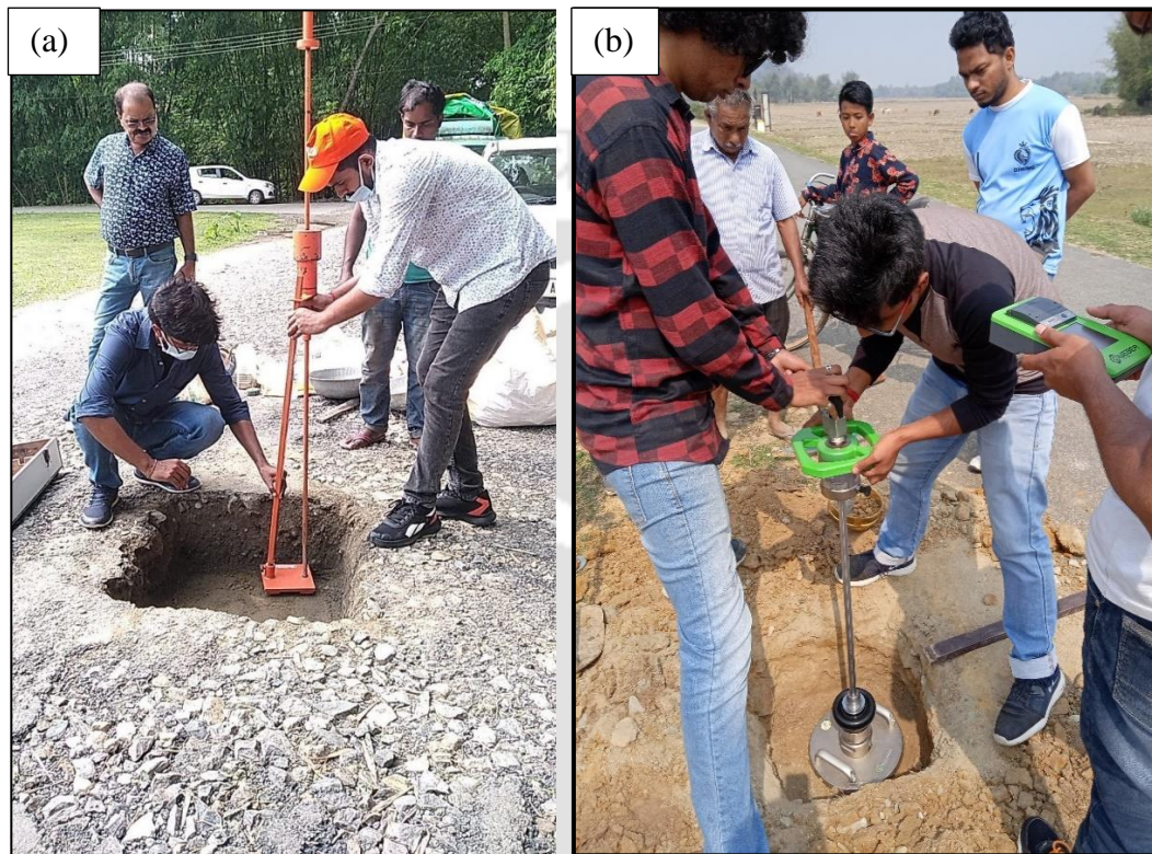
Figure 3.13: (a) Dynamic Cone Penetration test (b) Light Weight Deflectometer
