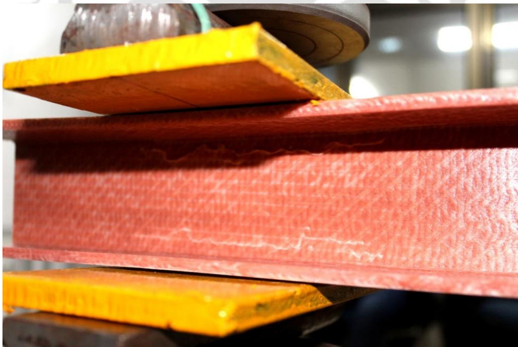
Figure 4.7(b): Failure modes of ITF-N70-tp10-1.
