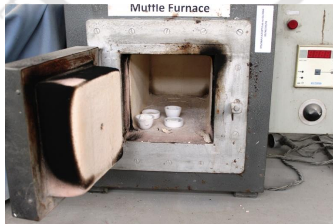
Figure 3.2: Muffle furnace with specimens.
