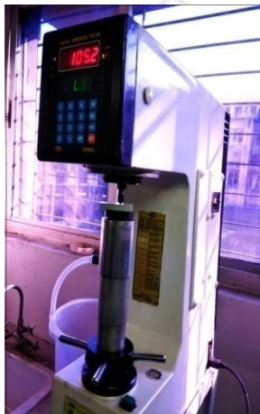
Figure 3.4: a) Rockwell hardness testing machine; b) hardness values for the GFRP profiles in L-scale .
