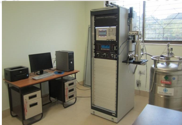
Fig. 2.10: Photographs of the RF impedance/material analyzer equipped with temperature control systems used to measure the dielectric properties.
