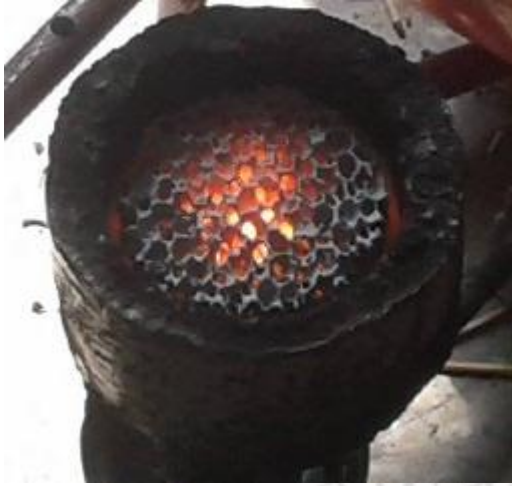
Fig. 4.9: Combustion of single layer of SiC.
