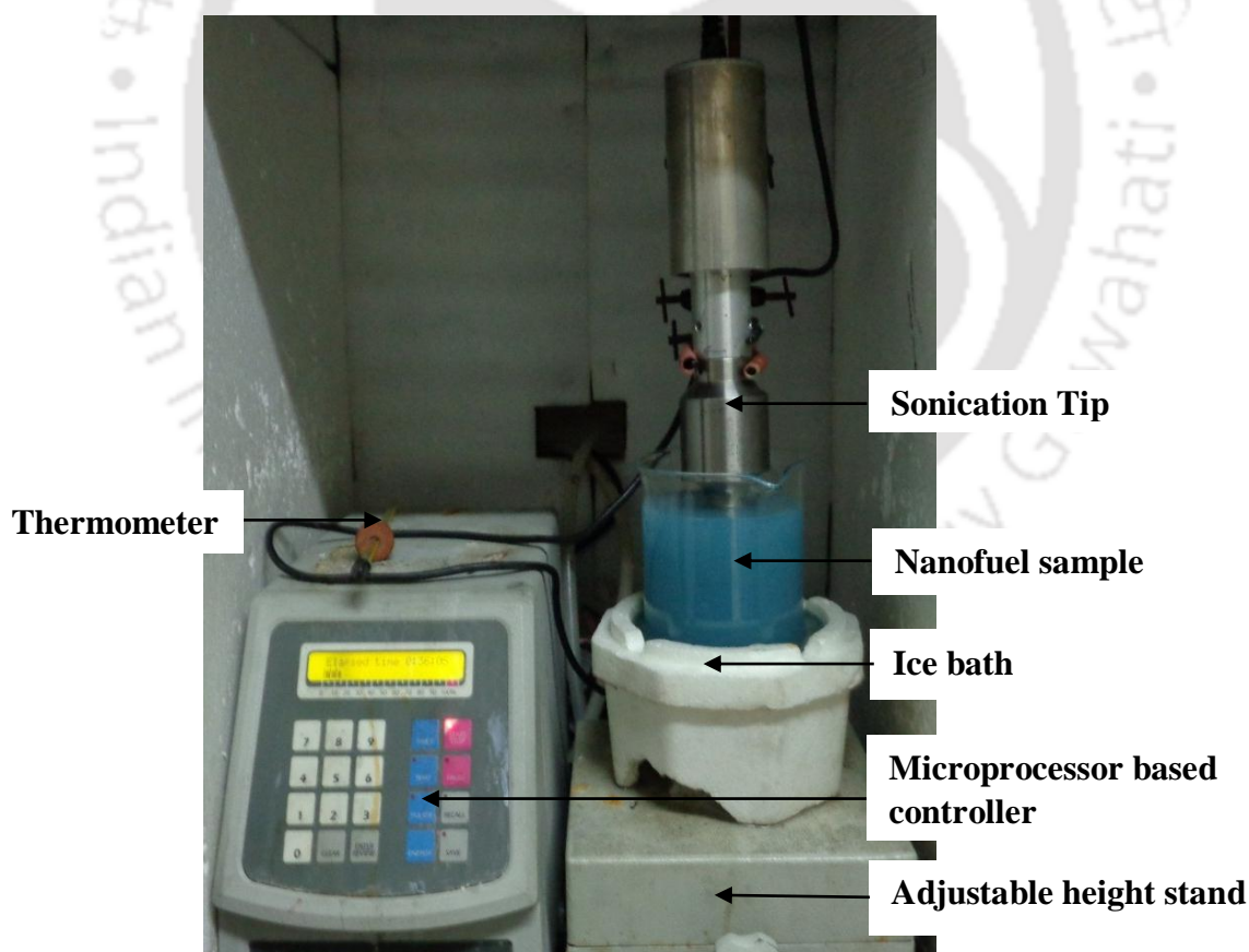
Fig. 5.1: Tip sonicator used to prepare nanofuel.
