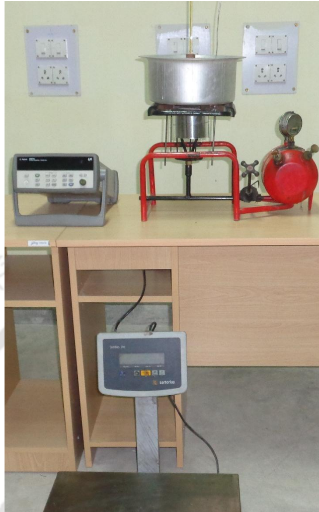
Fig. 6.13: Photographic view of experimental setup for measuring thermal efficiency.
