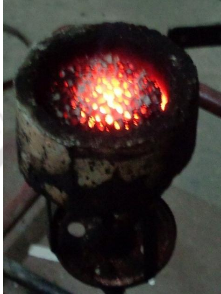
Fig. 4.11: Double layer of PM after combustion in cement casing.
