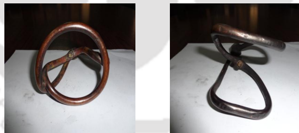
Fig. 3.9: (b) Different type of non-helical copper wire burner.
