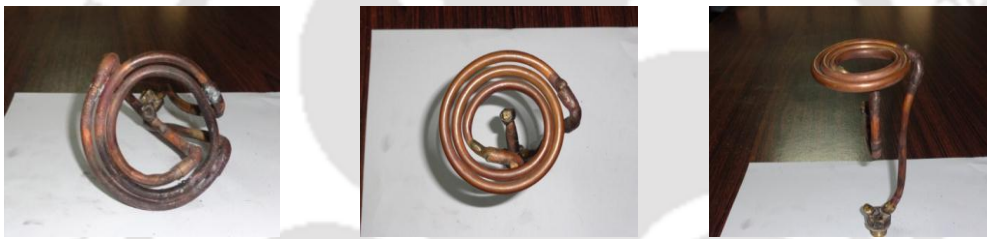
Fig. 3.9: (a) Different type of helical copper wire burner.
