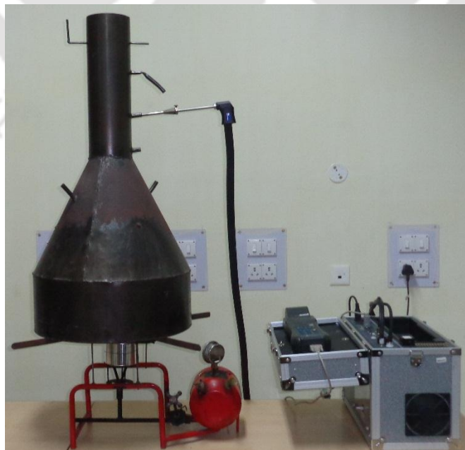
Fig. 6.14: Photographic view of experimental setup for measuring emissions.
