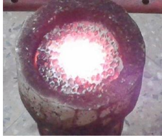
Fig.4.10: Combustion of single layer of SiC at higher pressure.
