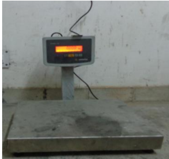
Fig.3.4: Strain gauge based weighing balance machine.
