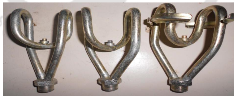
Fig. 3.12: Picture of the newly designed burners.
