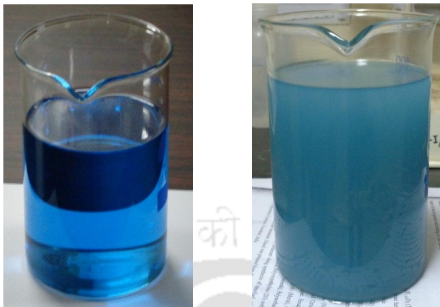
Fig. 5.2: Sample of pure kerosene and nanofuel prepared using tip sonicator.
