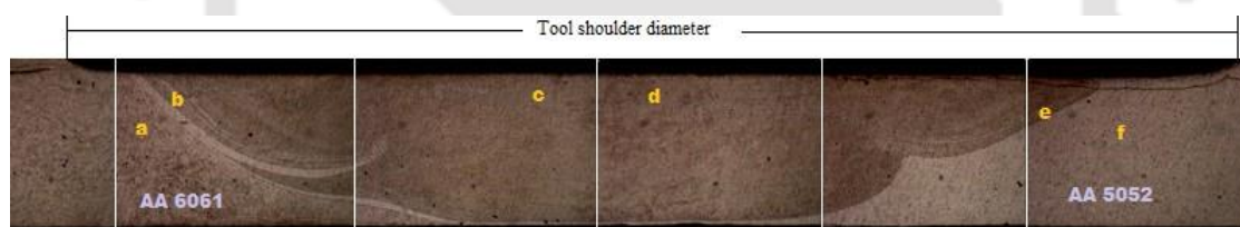
Fig. 4.8 Optical macrographs of the cross-section perpendicular to the tool traverse direction of FSW sample welded at 68 mm/min speed.
