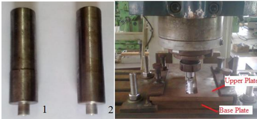
Fig. 3.2 Samples of the tools used & assembly of clamping fixture for FSW process.
