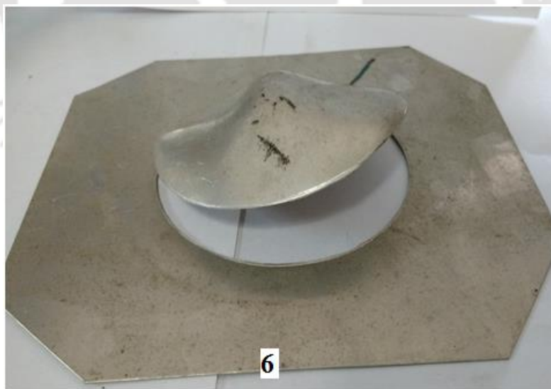
Fig. 6.9 Shearing of the blank at 12.88 kV.
