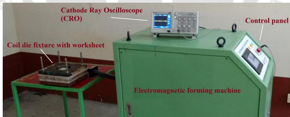
Fig. 3.5 The electromagnetic forming system.
