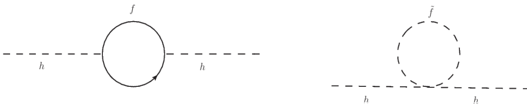
FIGURE 1.2: One-loop corrections to m_h^2 . Contributions from Dirac fermions (left) generate quadratically divergent terms in the expression of m_h^2 which are cancelled by contributions from scalar fermions (right) in supersymmetric models.
