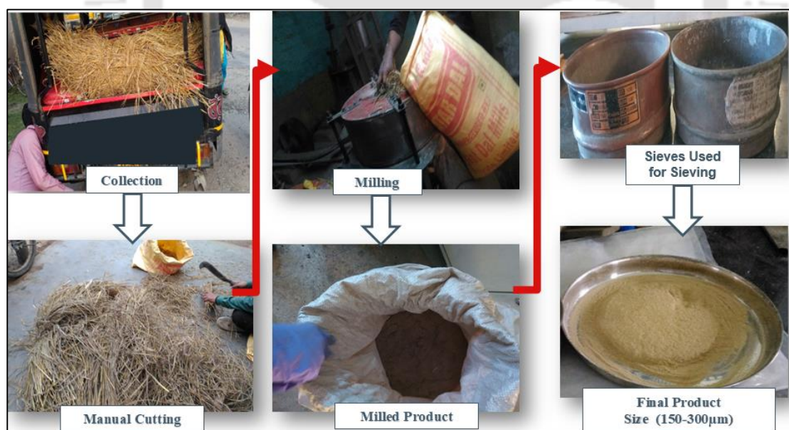
Figure 4.1. Rice straw collection and its pre-processing
