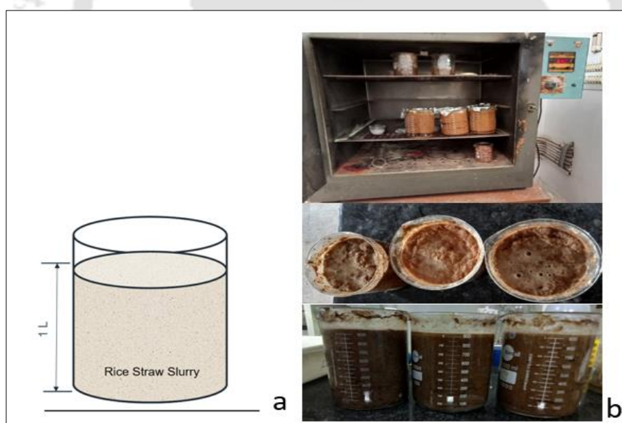
Figure 4.4.1. (a) Schematic diagram (b) Images of thermoalkali treated rice straw slurry
