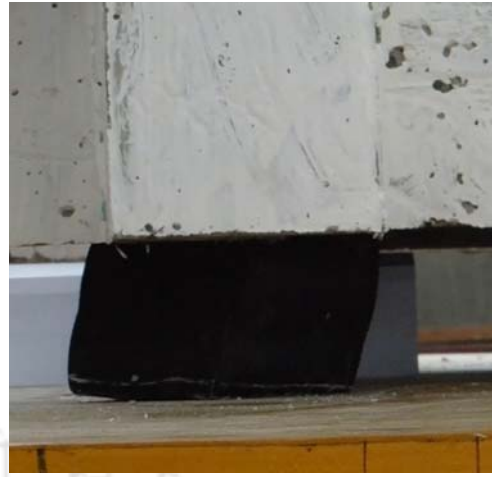
(b) 70% of PGA applied along 45^{\circ} to X-axis of FREI
