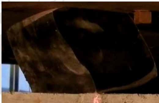
(f) at 60mm maximum displacement (45° loading direction)
