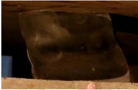
(c) at 30mm maximum displacement ( 0^{\circ} loading direction)
