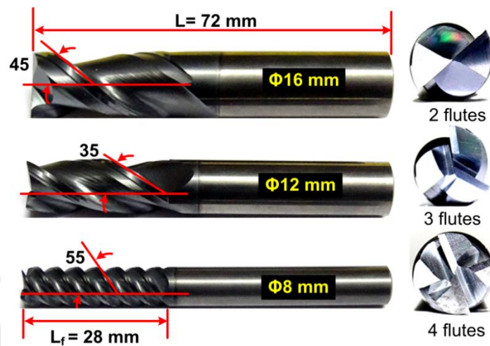
Figure 5.14 End milling cutters and tool geometry parameters
