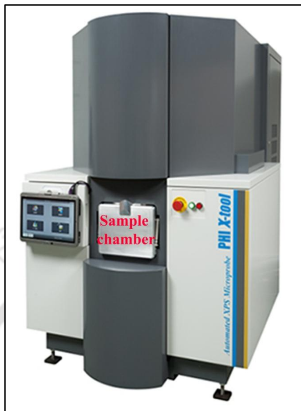
Fig. 2.9. Photograph of the X-ray photoelectron spectrometer (ULVAC-PHI, Inc.).
