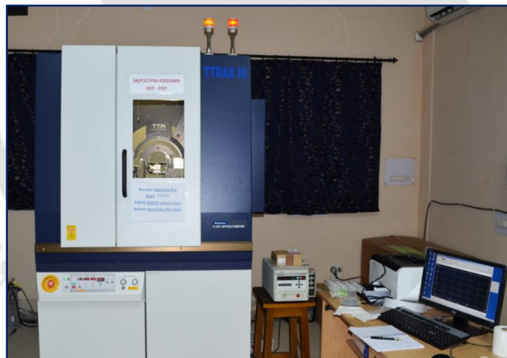
Fig. 2.8. A photograph of the X-ray Diffractometer (Rigaku RINT 2500, TTRAX III).
