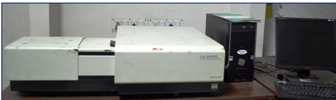
Fig. 2.11. A photograph of the UV-Vis-NIR spectrometer (Shimadzu, Japan).
