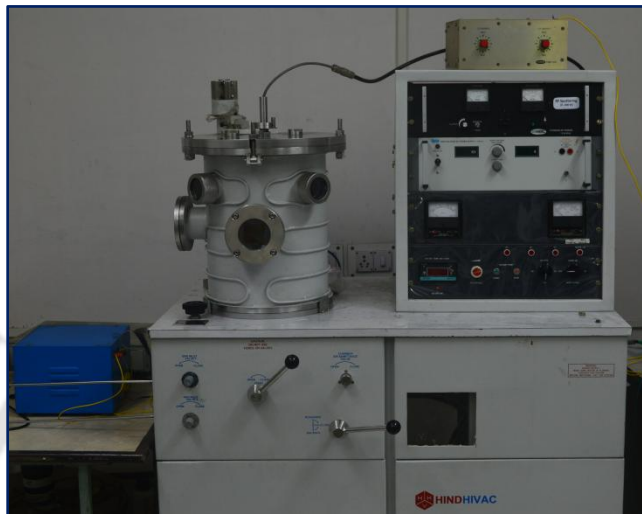
Fig. 2.4. A Photograph of the magnetron sputtering system (Hind Hivac, Bangalore).
