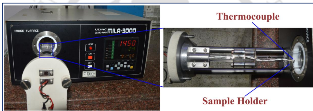
Fig. 2.2. A digital photograph of the RTA system (Mila 3000P, ULVAC, Japan).
