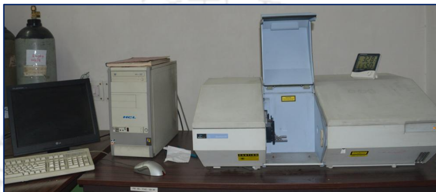
Fig. 2.10. A photograph of the FTIR spectrometer (Perkin Elmer, Spectrum BX).
