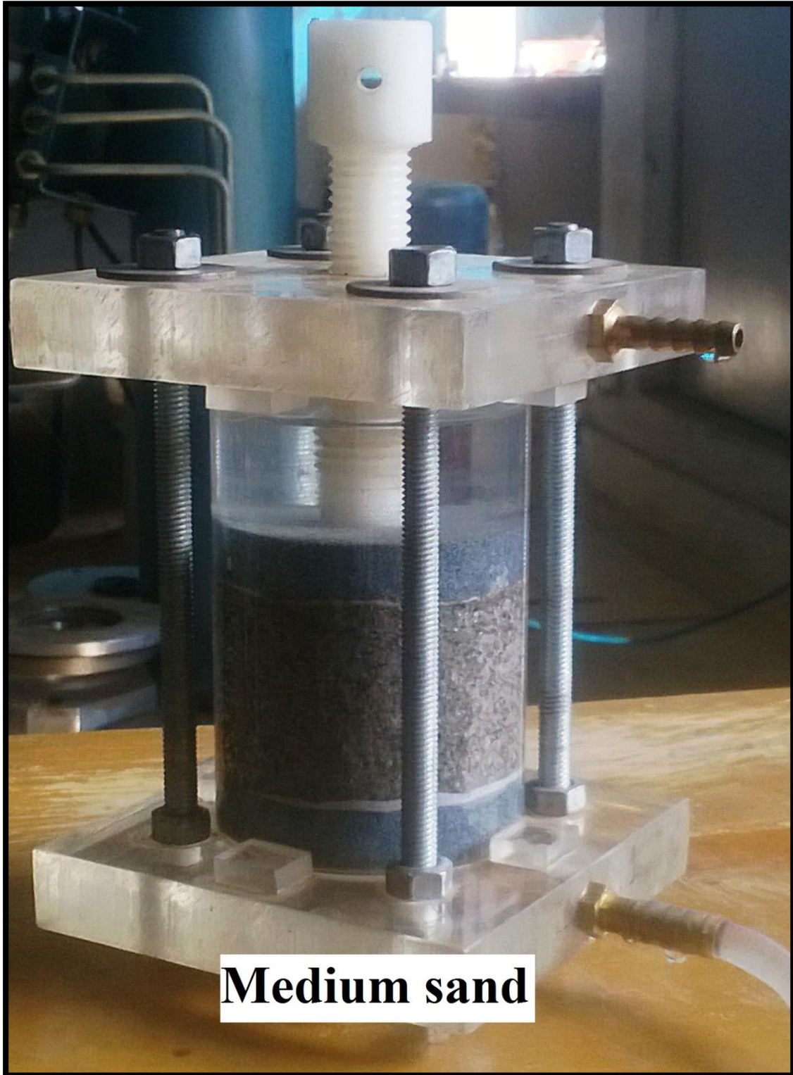
Appendix Figure M 1. 2: Permeability test mould showed Medium sand (thickness = 5 cm) setup used for the permeability test.
