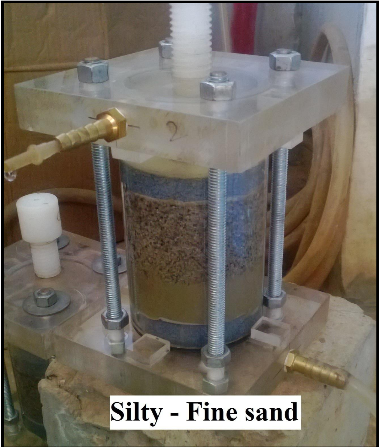
Appendix Figure M 1. 1: Permeability test mould showed a combination of clay (thickness = 2 cm) and Fine sand (thickness = 4 cm) setup used for the permeability test.
