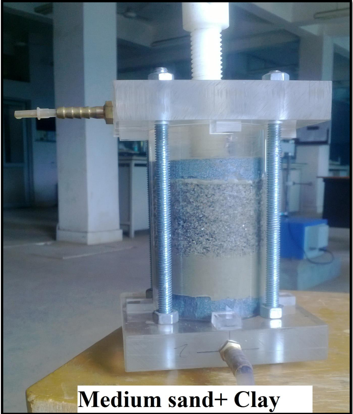
Appendix Figure M 1. 3: Permeability test mould showed Medium sand (thickness = 4 cm) and clay (thickness = 2 cm) setup used for the permeability test.
