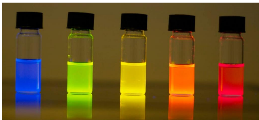
Fig 1.3 Wide range of emission color from CdSe/ZnS Qdots of different size. (Reprinted with permission from Reference [28]. Copyright ACS Nano 2014 American Chemical Society.)
