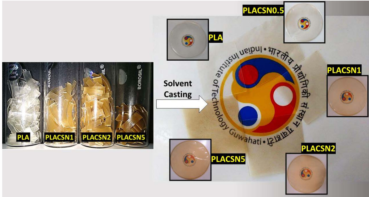
Figure 2.6: Fabrication of PLA and PLA/CSN films by solution casting method.
