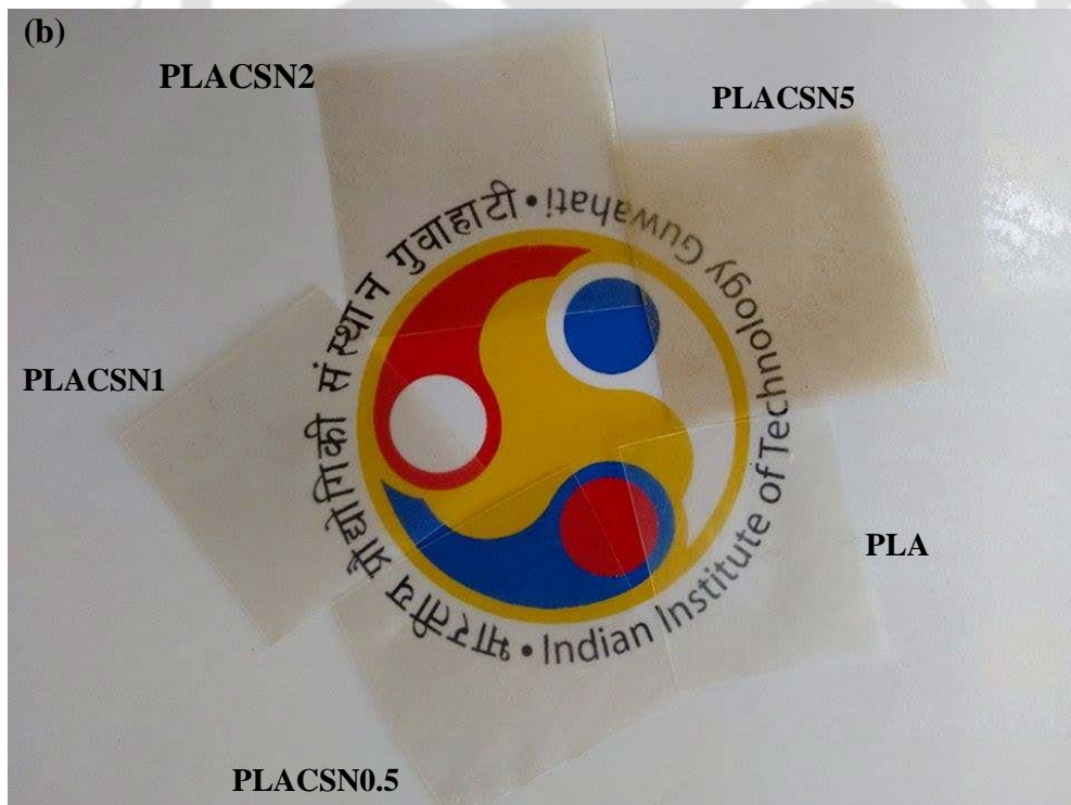
Figure 4.11: (a) Transparency, haze and color parameters, inset: greenness values and (b) visual photographs for PLA and PLA/CSN bionanocomposites.
