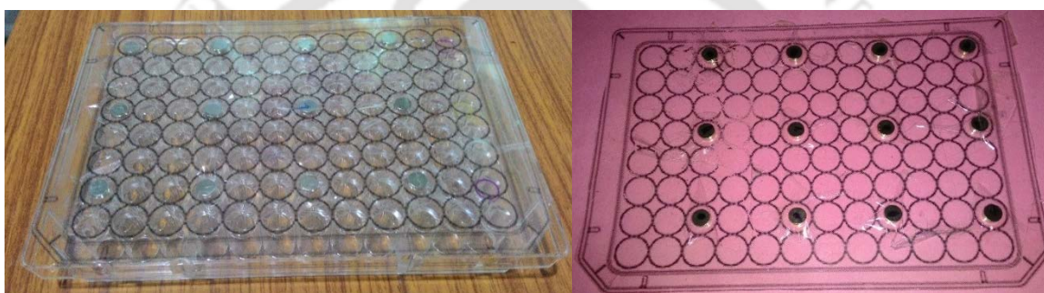
Figure 2.9: Twelve (12 nos.) neodymium magnets arranged onto 96-well culture plate.
