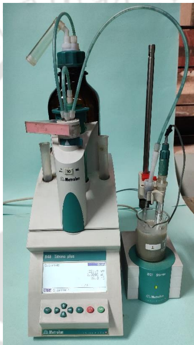
Fig. 3.9: Test setup for potentiometric titration using automatic titrator for determination of free and total chloride content
