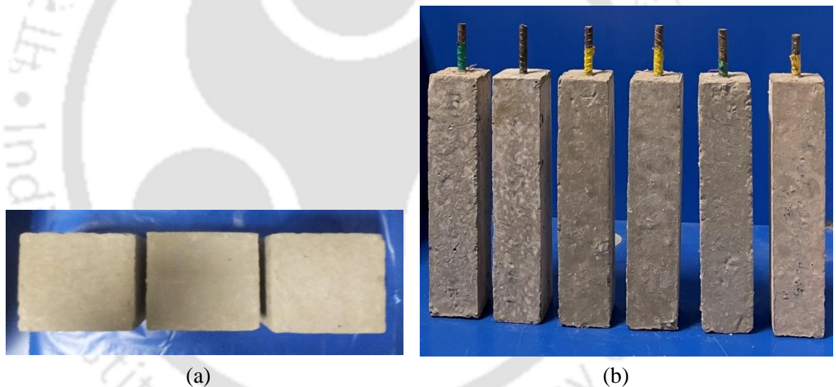
Fig. 3.6: Hardened GPC (a) cube specimens and (b) prismatic reinforced specimens
