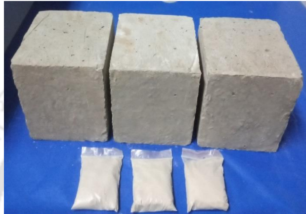
Fig. 3.7: GPC powder samples obtained from cube specimens
