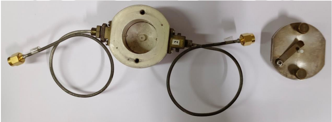
Figure 2. 18: QWED Krupka cavity resonator used for analyzing microwave dielectric properties of pure and composite AlN ceramics.
