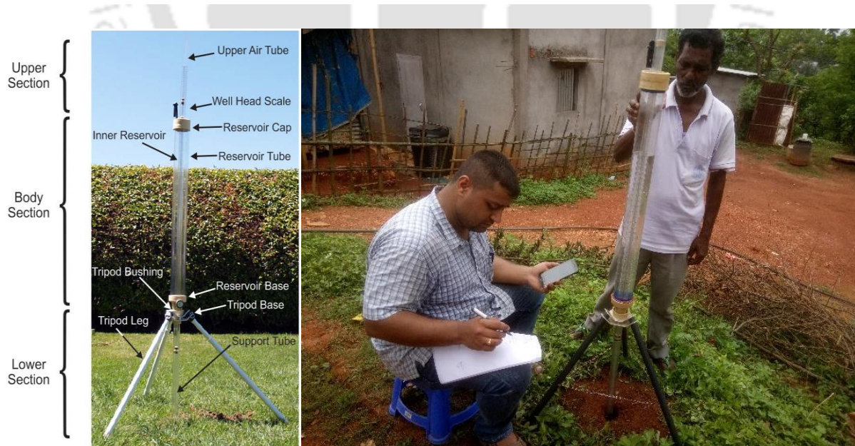
Figure 4.6 (a) Guelph Permeameter employing the Mariotte Principle (Guelph Permeameter Operating Instruction, 2008); (b) Guelph Permeameter test conducted in-situ
