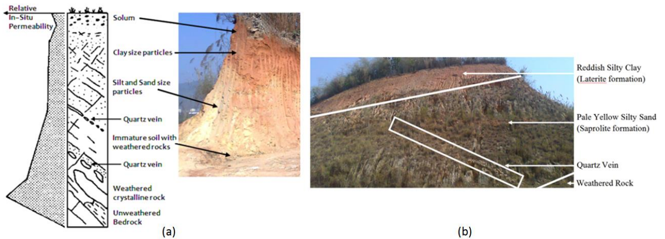
Figure 3.12 (a) Soil profile of a cut slope (from Selby, 1993) (b) soil profile of another cut slope at the IIT Guwahati Campus
