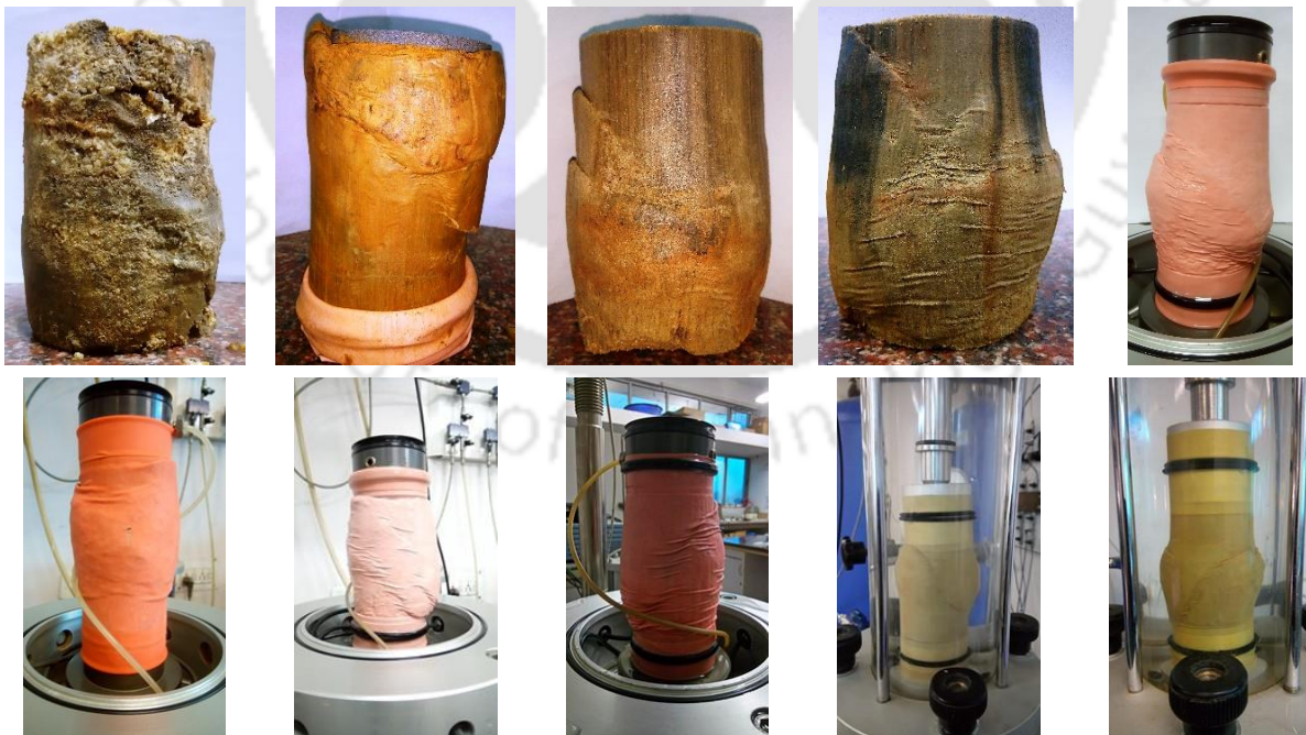
Figure 4.11 Sheared soil samples after triaxial test
